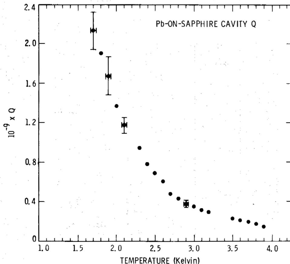
Fig. 1. Quality factor  $Q$  of a Pb-on-sapphire resonant cavity with resonant frequency of 2.69 GHz.
