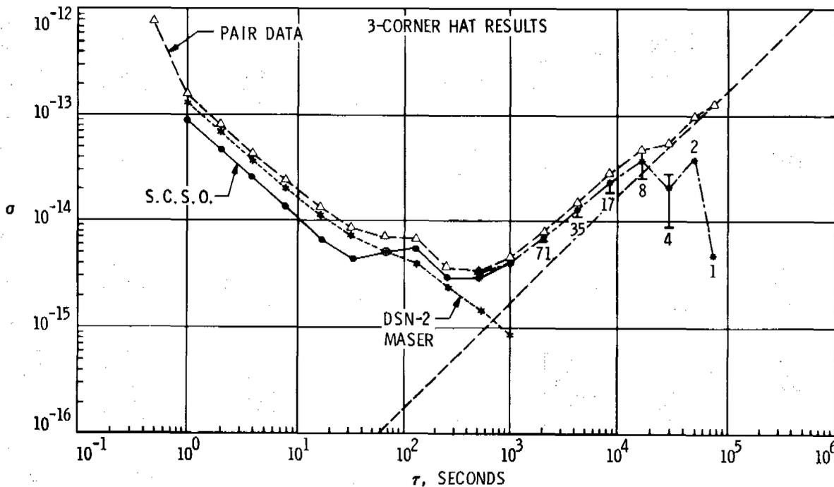
Fig. 3. Allan variance of frequency fluctuations for the superconducting cavity stabilized oscillator (SCSO), measured versus two hydrogen masers in a three-corner hat technique. The SCSO is the comparison oscillator used to characterize our superconducting cavity maser (SCM) oscillator.
