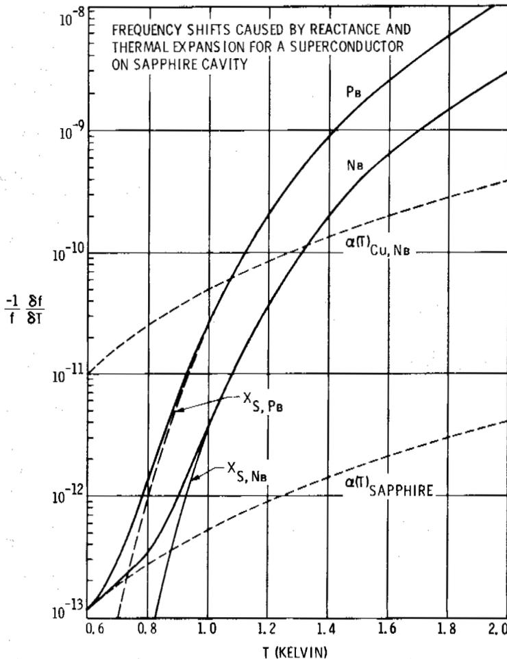
Fig. 5. Relative frequency shifts  $[-1/f]\delta f/\delta T$  caused by temperature fluctuations in a superconductor on sapphire cavity, at temperatures indicated on the abscissa.
