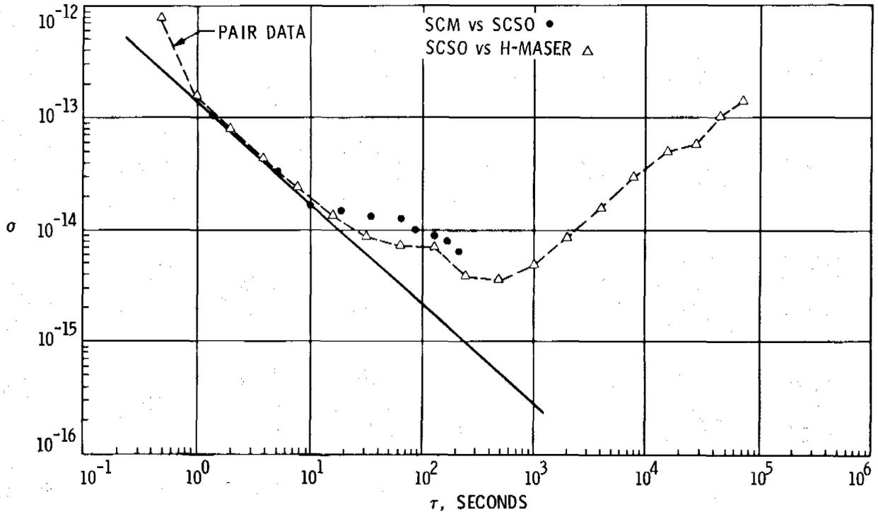
Fig. 4. Allan variance of frequency fluctuations for the superconducting cavity maser (SCM) oscillator, measured versus the SCSO. The triangles show, for comparison, the pair data for the SCSO versus the Hydrogen Maser. The solid line represents the limiting resolution of the data gathering system.
