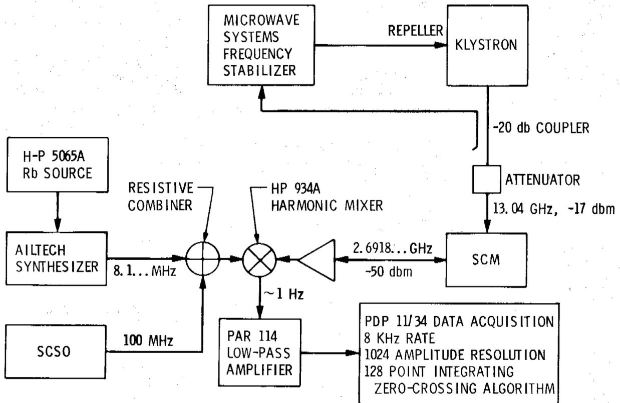
Fig. 2. Block diagram of the data gathering system used to measure Allan variance values of frequency fluctuations. Typical signal frequencies and amplitudes are indicated.
