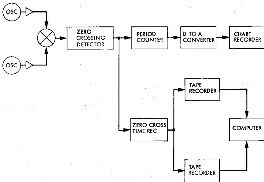
Fig. 7. Frequency Stability Instrumentation Block Diagram
