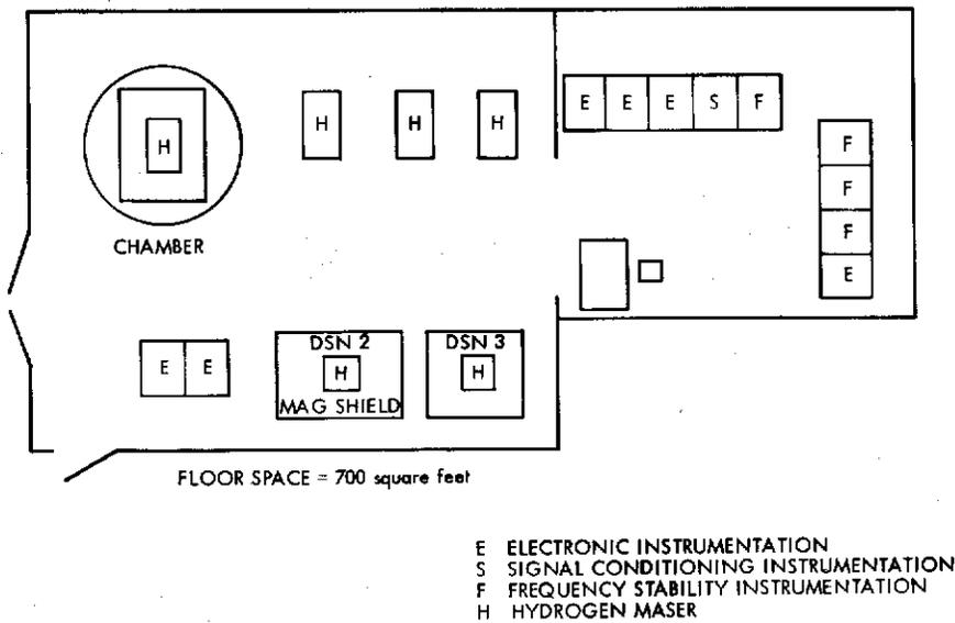
Fig. 6. Frequency Standard Test Laboratory Floor Plan
