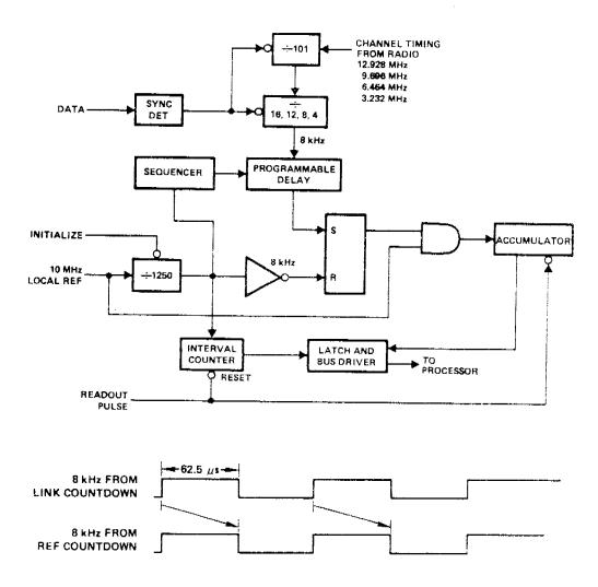
Figure 3. Phase Detector and Example Measurement
