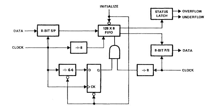
Figure 6. 1024-Bit Elastic Buffer
