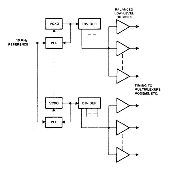
Figure 5. Frequency Synthesizers and Distribution Amplifiers
