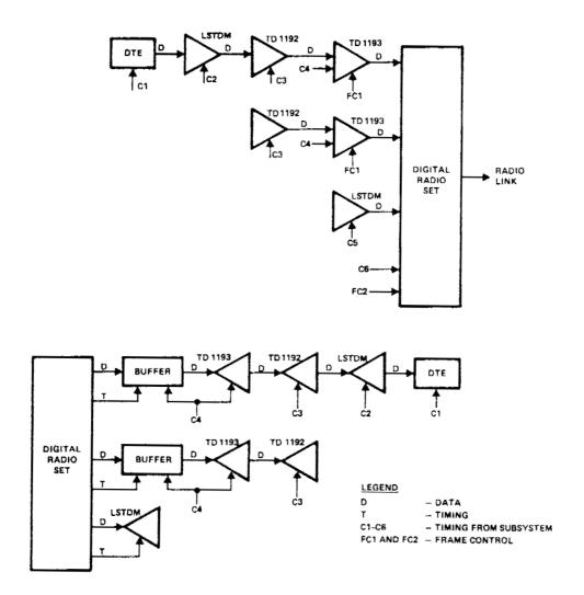
Figure 1. Transmit and Receiver Configurations
