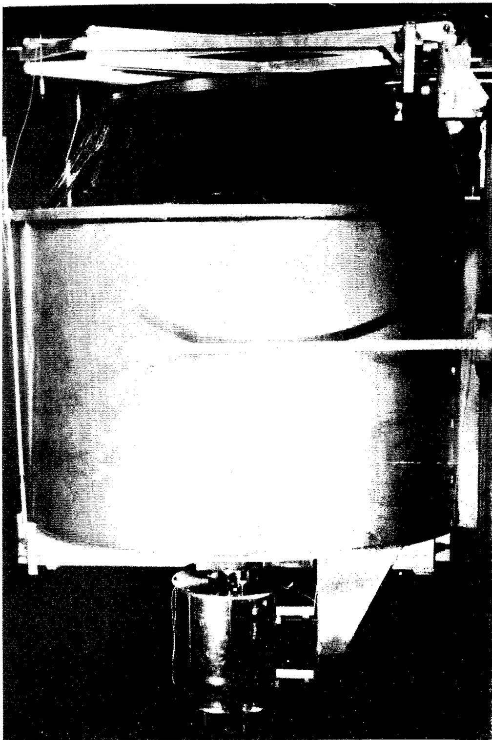
Figure 2. Flexible Cone-Large Storage Box Hydrogen Maser
