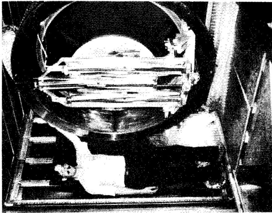
Figure 3. Flexible Cone and Drive
