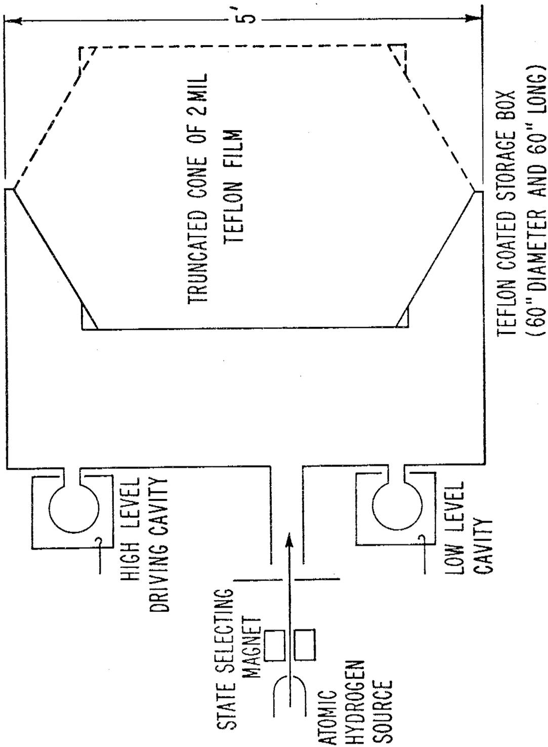
Figure 1. Schematic Diagram of the Large Storage Box Maser with Flexible Box
