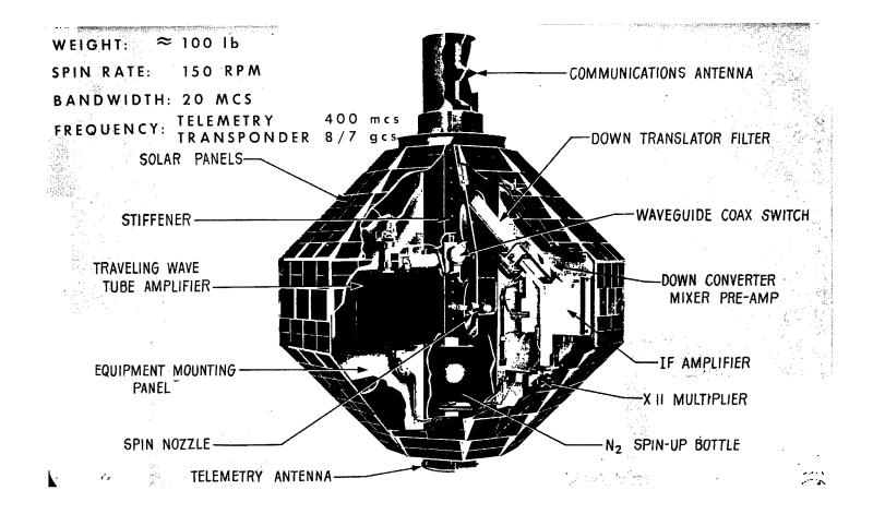
Figure 1. SPACE SUBSYSTEM - SATELLITE
