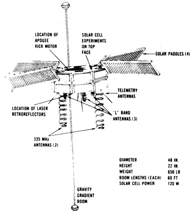
Fig. 8. Timation III or NTS-1 satellite. Timation II for which measurement results are reported has a similar outer appearance.
