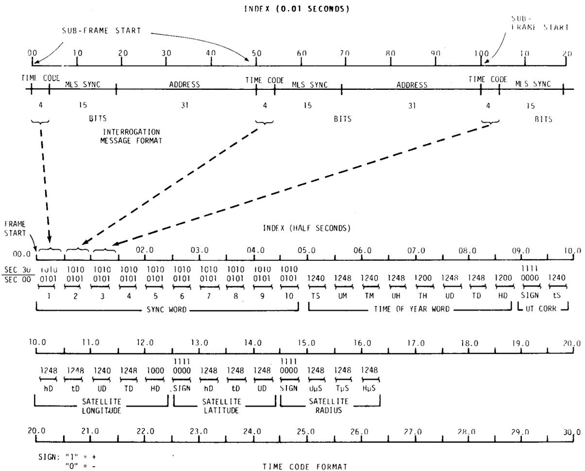
Fig. 6. SMS time-code format and multiplexing into SMS interrogation channel.
