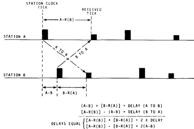
Fig. 16. Principle of simultaneous duplex time transfer.
