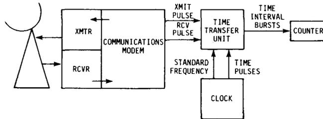
Fig. 17. Configuration for time transfer using modems.
