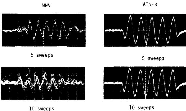
Fig. 3. Multiple oscilloscope sweeps of the WWV and ATS-3 ticks.
