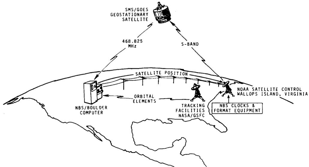
Fig. 5. SMS time-code distribution system.
