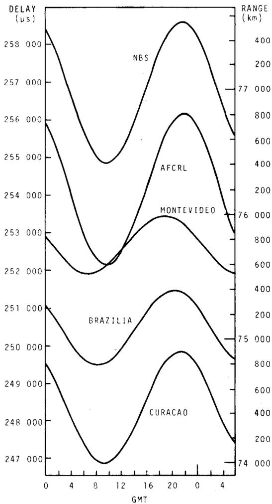
Fig. 2. Delay variation due to satellite motion (AFCRL = Air Force Cambridge Research Laboratory).
