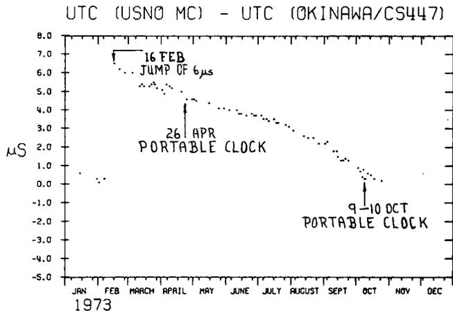
Fig. 19. Time transfer between USNO and Okinawa via DSCS.
