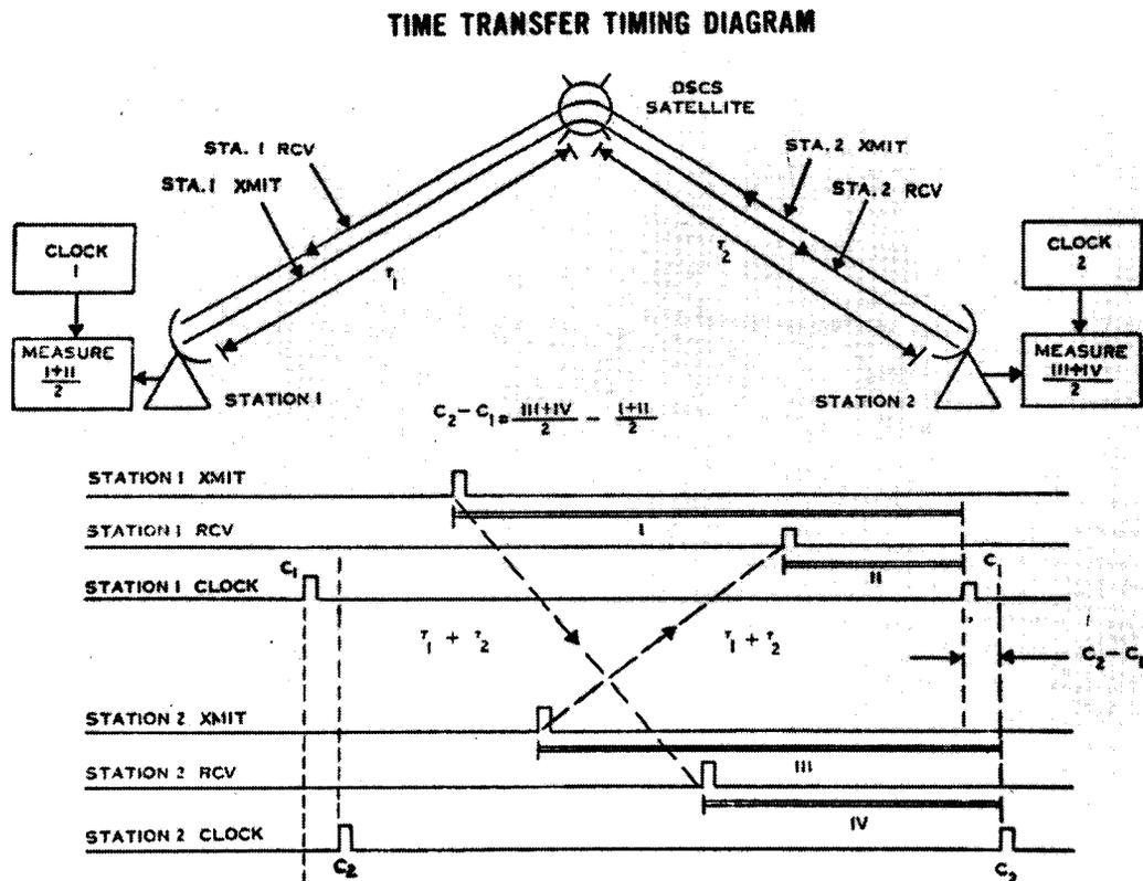
Fig. 15. Time transfer via satellite relay (round trip).
