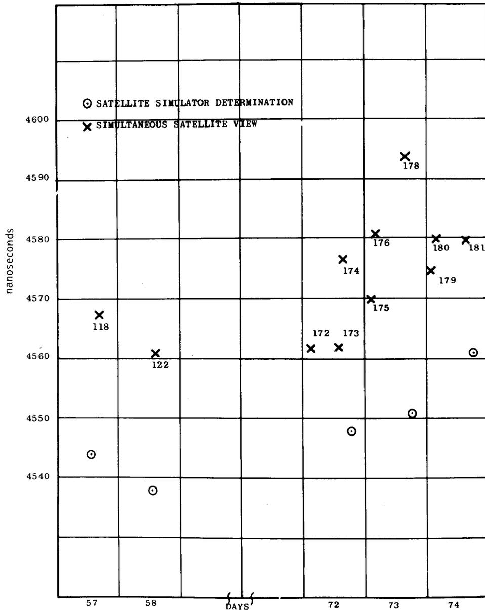
Fig. 12. Regional clock-synchronization data using the Transit system.
