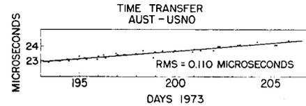
Fig. 9. Time transfer between USNO and Australia via Timation II.
