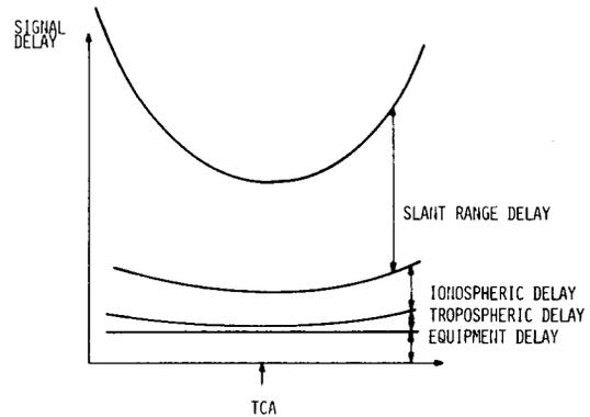
Fig. 10. Clock synchronization method.
