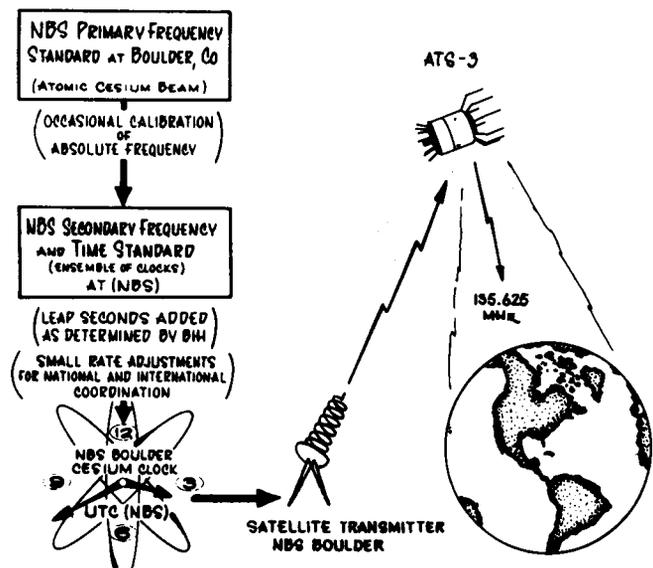
Fig. 1. Time and frequency broadcasting from the ATS-3 satellite.
