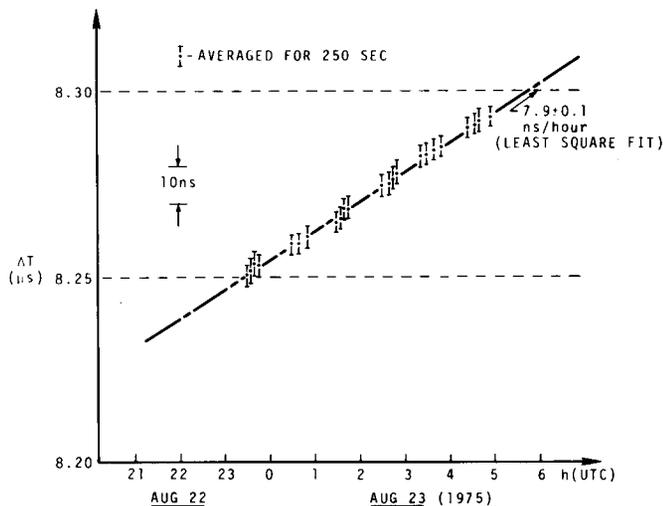
Fig. 20 Example of measured time difference via ATS-1  $\Delta T$  = reference clock (Kashima, RRL)—reference clock (Rosman, NASA).
