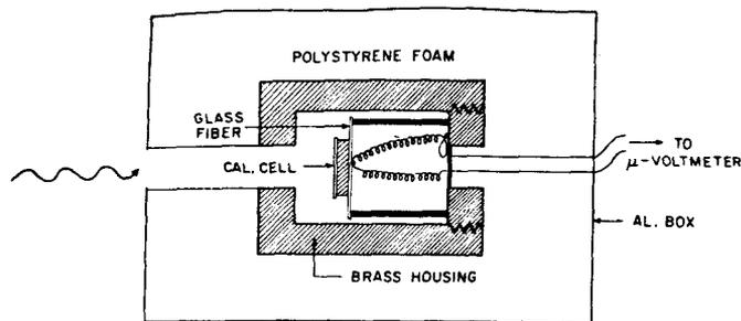
Fig. 1. Cross-sectional diagram of the calorimeter, showing layout of components, method of supporting calorimeter absorption cell, and position of the thermocouple.
