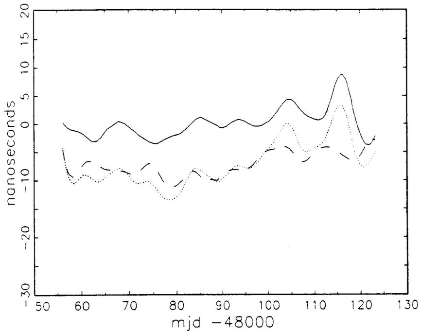
FIGURE 6: Difference between the corrected and the raw values UTC(OP) - UTC(NIST). The corrected values UTC(OP) - UTC(NIST) are obtained with:
