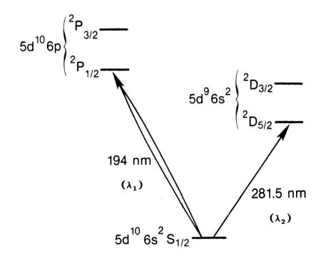
Fig. 1. Electronic energy levels of  $Hg^{\dagger}$ . The ground electronic state of the <sup>199</sup> $Hg^{\dagger}$  isotope is made up of two hyperfine levels, separated by 40.5 GHz. Some microwave frequency standards are based on this transition. An optical frequency standard might be based on the 281.5 nm transition.
