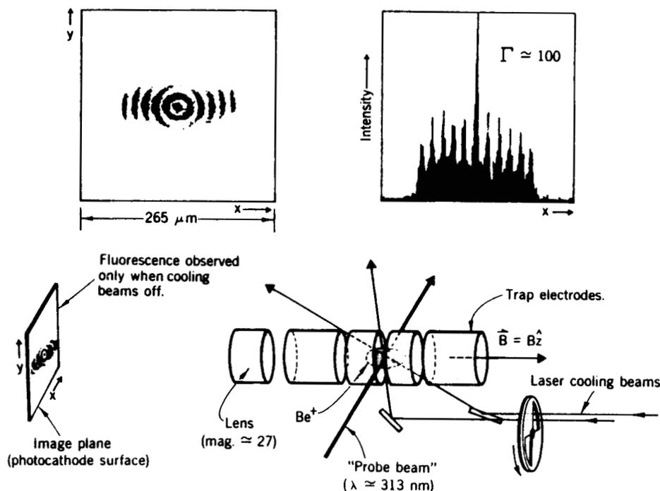
Fig. 5. Schematic representation of apparatus for observation of shell structure of strongly coupled  $^9Be^+$  ions in a Penning trap. Images are made of the ions which are intersected by the probe beam. In the upper right, an intensity plot vs x for a value of y intersecting the center of the cloud is shown. Shell structure results from the boundary conditions at the edge of the cloud.
