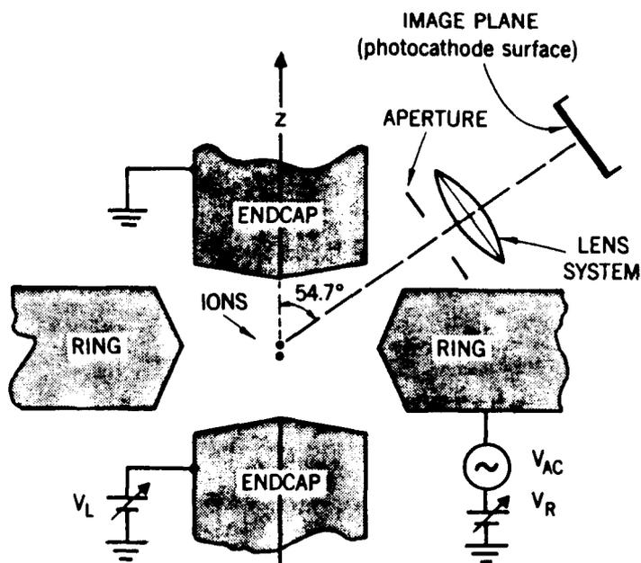
Fig. 3 Schematic drawing of the trap electrodes (to scale) and imaging system (not to scale) for  $\text{Hg}^+$  cluster experiments. The end-cap to end-cap separation along the  $z$  axis is approximately  $625 \mu\text{m}$ . The overall magnification of the lens system is 180X. The laser beam used to illuminate the ions also enters the trap at an angle of  $54.7^\circ$  with respect to the  $z$  axis and is perpendicular to the observation axis shown.
