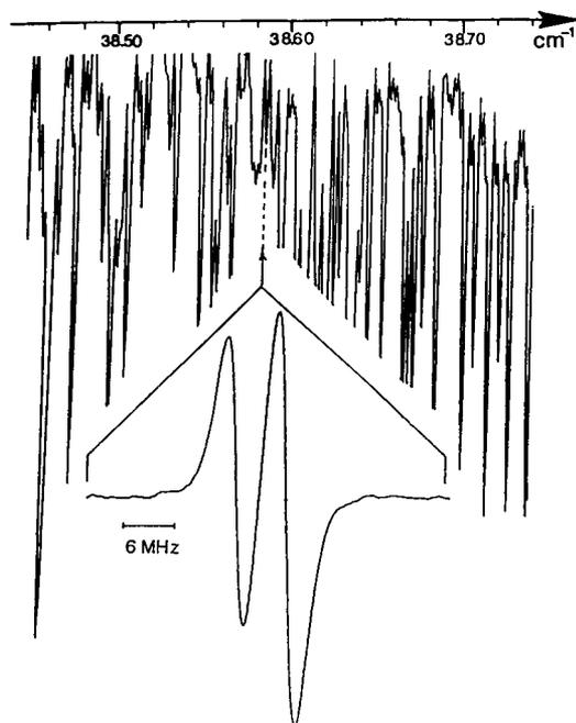
FIG. 1. Resolution of TuFIR vs a Fourier transform spectrum. The doublet corresponding to the (26, 6)-(26, 5) transition, which is collapsed into a single line in the FTS spectrum, is still clearly resolved.
