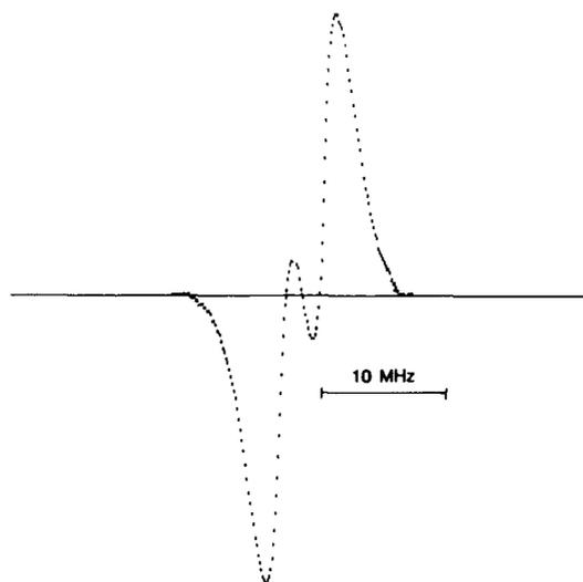
FIG. 3. The line doublet corresponding to the (28, 5)–(27, 5) transition. A partial overlapping of the dispersion-shaped curves decreases the accuracy of this measurement.
