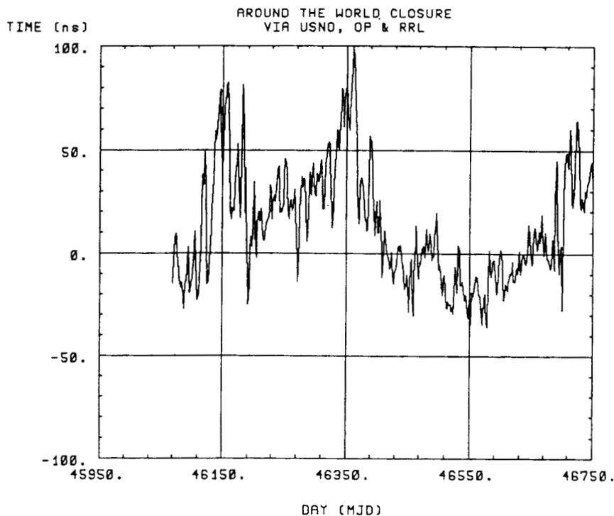
**Fig. 4.** Residuals after transferring time via GPS satellites in common view around the world for about two years using USNO in Washington D.C., USA, OP in Paris, France, and RRL in Tokyo, Japan as pivots. MJD 46066 is January 1, 1985, and MJD 46431 is January 1, 1986
