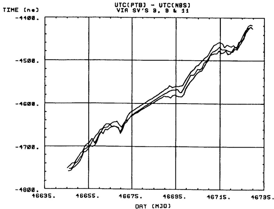
Fig. 1. Biases between different SVs used in common view between PTB in Europe and NBS in Western North America
