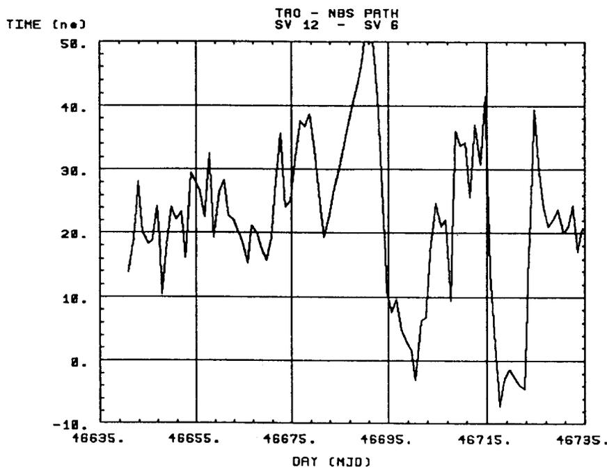
Fig. 2. Differences of TAO-NBS Japan to Western North America common-view data via SV 12 minus SV 6 showing the bias between them. The mean bias is 22.4 ns
