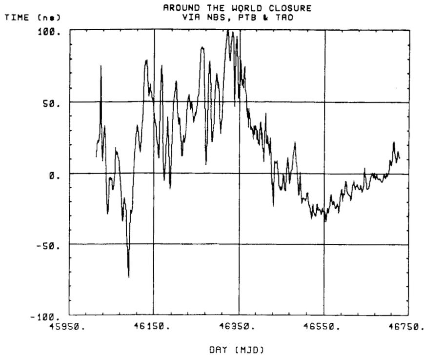
**Fig. 3.** Residuals after transferring time via GPS satellites in common view around the world for about two years using NBS in Boulder, Colorado, USA, PTB in Braunschweig, W. Germany, and TAO in Tokyo, Japan as pivots. MJD 46066 is January 1, 1985, and MJD 46431 is January 1, 1986
