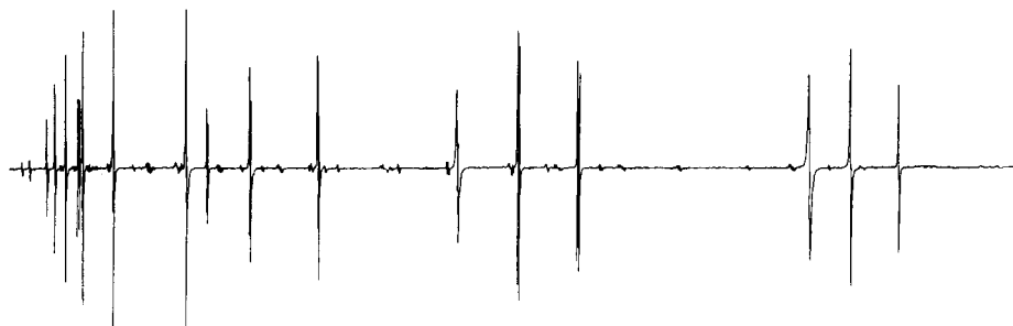
FIG. 1. The LMR spectrum of chromium hydride ( \text{CrH } X^6\Sigma^+ ) associated with the N = 3 \leftarrow 2 transition, recorded with the 1100.8067 GHz laser line of \text{CH}_2\text{F}_2 ( 272.3 \mu\text{m} ) in \pi polarization. The scan is from 0–1 T with a time constant of 0.1 sec.
