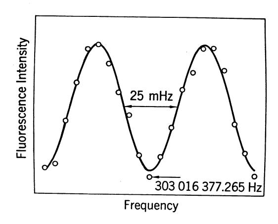
FIG. 2. Signal obtained with two 0.5s Ramsey pulses separated by a 19 s free precision interval on the clock transition in  $^9\mathrm{Be}^+$  (see text). The sweep width was 100 mHz and the frequency interval between points was 5 mHz. The dots are experimental and are the average of 10 sweeps; the curve is a least squares fit.
