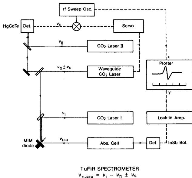
FIG. 1. Block Diagram of TuFIR spectrometer.
