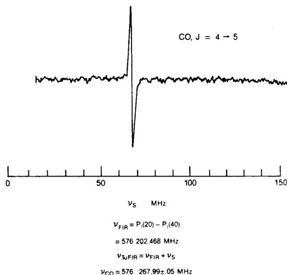
FIG. 2. CO absorption derivative signal for the  $J = 4-5$  transition of CO. Data were taken with a CO pressure of 5.3 Pa and a time constant of 400 ms.
