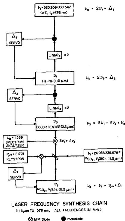
Fig. 1. At the top of the chain, a cw dye laser is locked to an  $\text{I}_2$  transition. A 1.15- $\mu\text{m}$  He-Ne laser is locked to the dye laser, and a 2.3- $\mu\text{m}$  color-center laser is locked to the He-Ne laser. The beat between the  $\text{CO}_2$  lasers and the color-center laser is measured.
