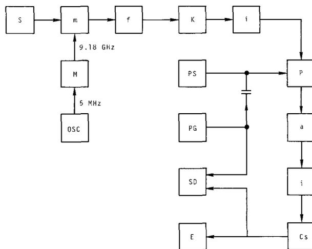
Fig. 1. Block diagram of the measurement system. S = frequency synthesizer, Osc = crystal oscillator, M = frequency multiplier (x 1836), m = mixer, f = filter, K = klystron, i = isolator, p = pin-diode switch, a = attenuator, Cs = cesium beam tube, PS = power supply (pin-diode bias), PG = pulse generator, SD = synchronous detector, E = electrometer
