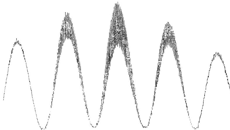
Fig. 3. Spectrum of the beam tube under pulsed operation:  $T = 1.8$  ms,  $\tau_p = 45$   $\mu$ s. The vertical scale is arbitrary. Other recording data are the same as in Fig. 2
