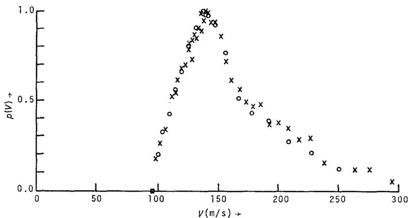
Fig. 7. Velocity distribution of the beam tube. Crosses are obtained with  $\tau_p = 45$   $\mu$ s, circles with  $\tau_p = 15$   $\mu$ s. The distribution function is normalized to 1.0 at the peak
