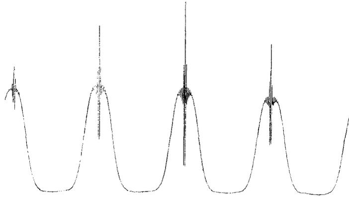
Fig. 2. Spectrum of the beam tube under normal cw operation. The separation between the main peaks is about 40 kHz. The sweep speed was 50 Hz/s. The recording time constant was 0.1 s. The vertical scale is arbitrary
