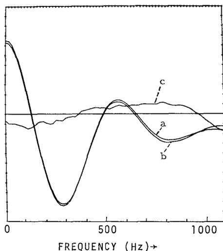
Fig. 8. Comparison of the experimentally measured Ramsey pattern under normal, cw operation (a) with a pattern (b) which was numerically calculated from Fig. 7. Zero on the frequency scale is the center of the Ramsey pattern. Also depicted is the difference (c) between these two curves using a magnification factor of 4
