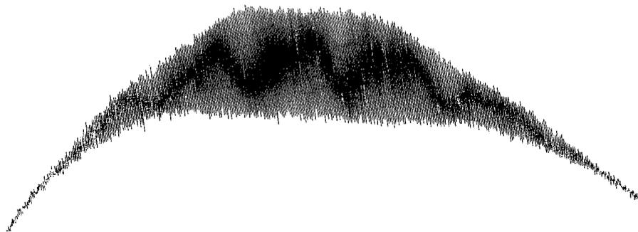
Fig. 4. Spectrum of the beam tube under pulsed operation:  $T = 1.8$  ms,  $\tau_p = 15$   $\mu$ s. Other recording data are the same as in Fig. 2. The short pulses do not allow resolution of the different transitions at the given magnetic field setting
