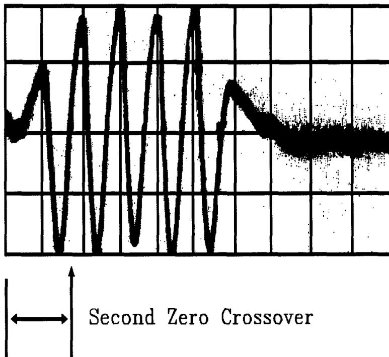
To further increase the resolution of delay measurement, increase the oscilloscope sweep rate to 100 microseconds per division and adjust the trigger pulse from the generator to be approximately 500 microseconds less than the total delay time previously measured. At these settings, the second zero crossover of the tick will be somewhere near the middle of the oscilloscope face.
