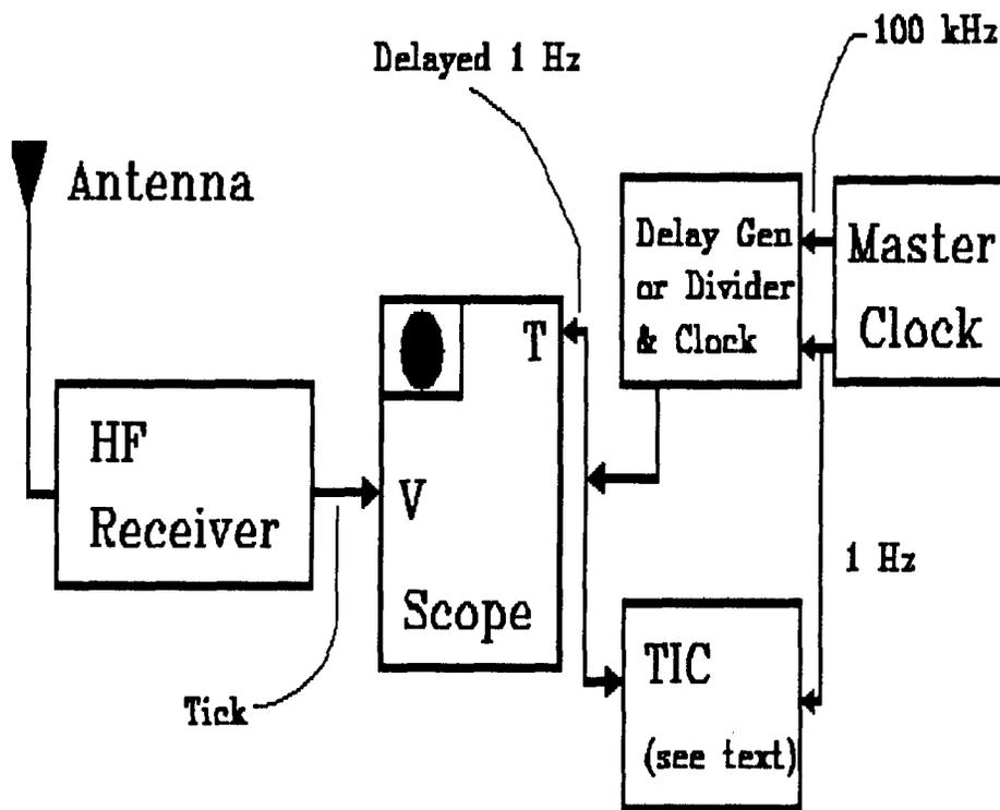
With the oscilloscope sweep adjusted to 1 millisecond per division, the trigger pulse should be delayed by an amount equal to the propagation delay in milliseconds. Don't worry about fractional milliseconds in the delay. The sweep should be adjusted so that it begins exactly at the left end of the horizontal graticule and is vertically centered.
