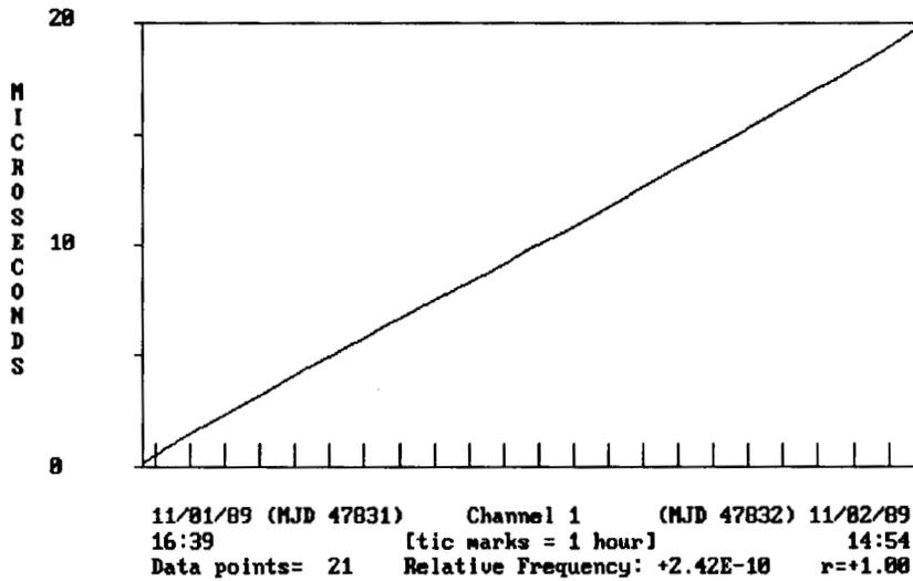
Cesium Oscillator vs Loran-C 9940 (Fallon, Nevada)
