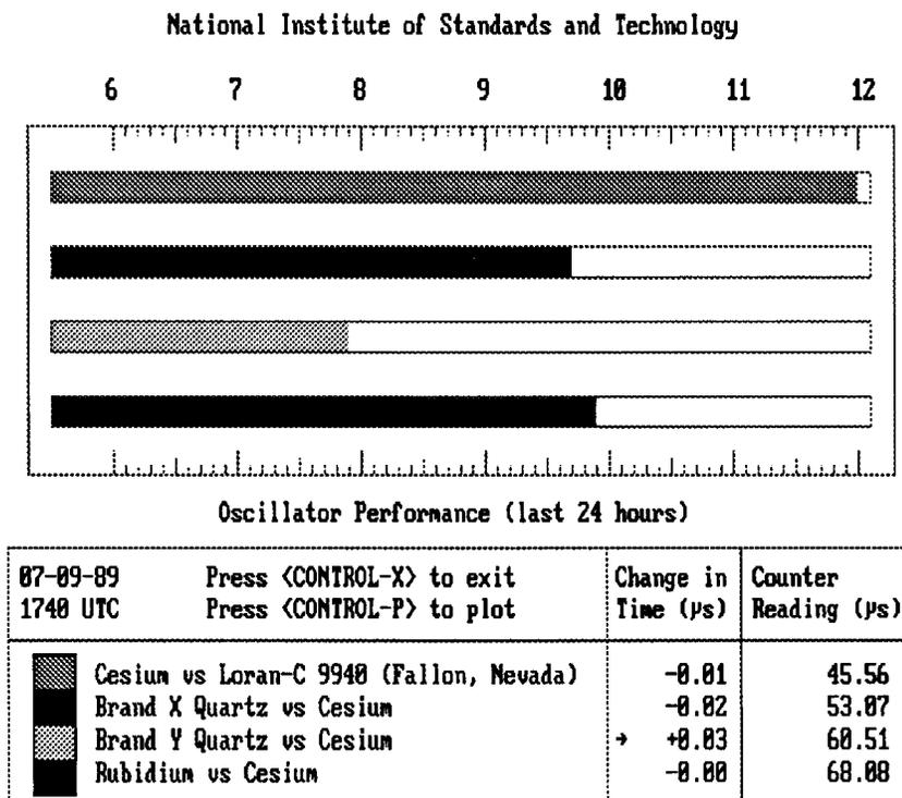
The measurement screen is divided into two parts. The bottom part of the screen contains a box with information about the signals being measured. The left side of this box shows the present time (UTC) and date. Below the date and time are the titles given to each measurement channel. On our sample screen (on the previous page) the title for Channel 1 is: Cesium vs Loran-C 9940 (Fallon)
