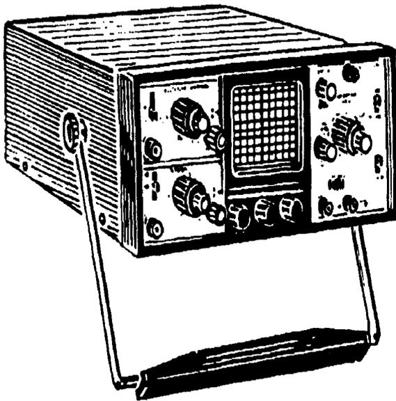
Recovering time at higher accuracies requires using electronic equipment. For example, if an oscilloscope is used to see the seconds ticks, the user can set clocks with much greater accuracy than is possible by only listening to the ticks.
