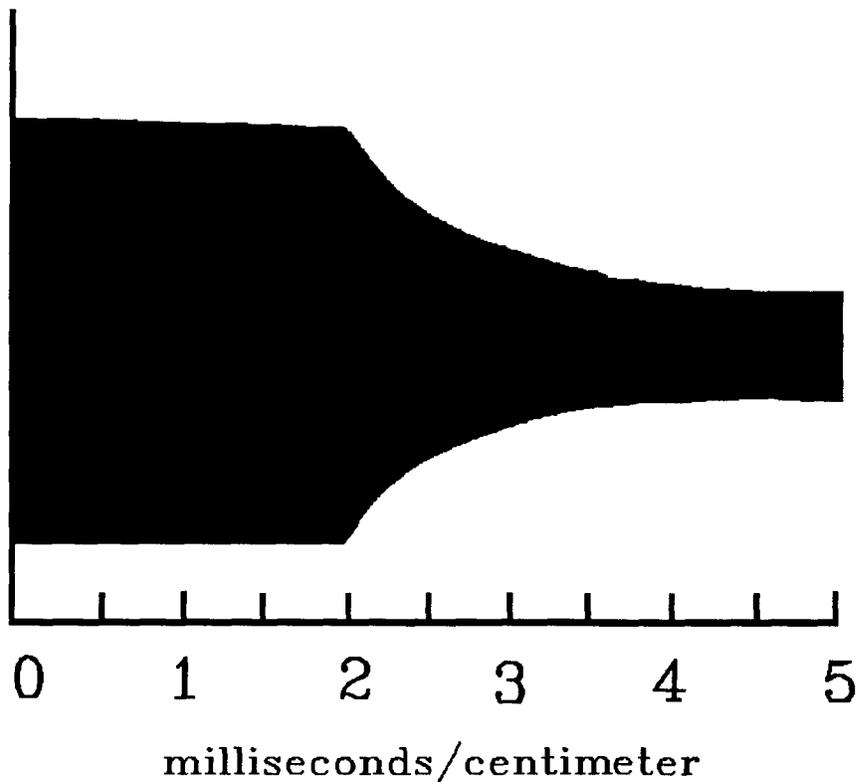
The actual process of time recovery consists of viewing the signal envelope on an oscilloscope that is being triggered by a local clock at the receiving site. Having previously determined the path delay, its value can be subtracted from the total observed delay on the oscilloscope to obtain the local clock error.
