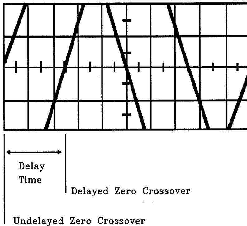
Without touching any of the oscilloscope controls, disconnect the 1-kHz signal from the vertical input and replace it with the delayed 1-kHz signal from the receiver output. Since a receiver delay is almost always less than 1 millisecond (1 cycle of a 1-kHz signal), there is little chance of ambiguity on which cycle to measure. The delay is equal to the sweep time from the reference undelayed crossover to the first delayed crossover point.
