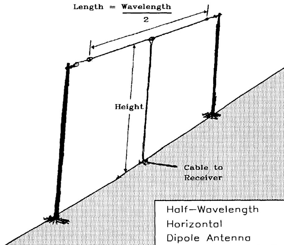
For nighttime reception on paths up to several thousand miles, the skywave is predominant, and a horizontal dipole half-wavelength antenna is recommended. The antenna should be located a quarter-wavelength or higher above ground. Choose an area free from obstructions and interference.
