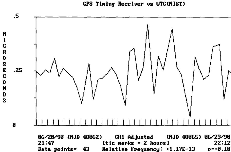
The plot shows data obtained with a commercially available GPS timing receiver. These receivers are readily available, and their cost has gone down over the past few years. The receiver was using the (C/A) code with intentionally degraded accuracy. Even so, the range of the data is less than 0.5 microsecond (500 nanoseconds) over the 3-day period.
