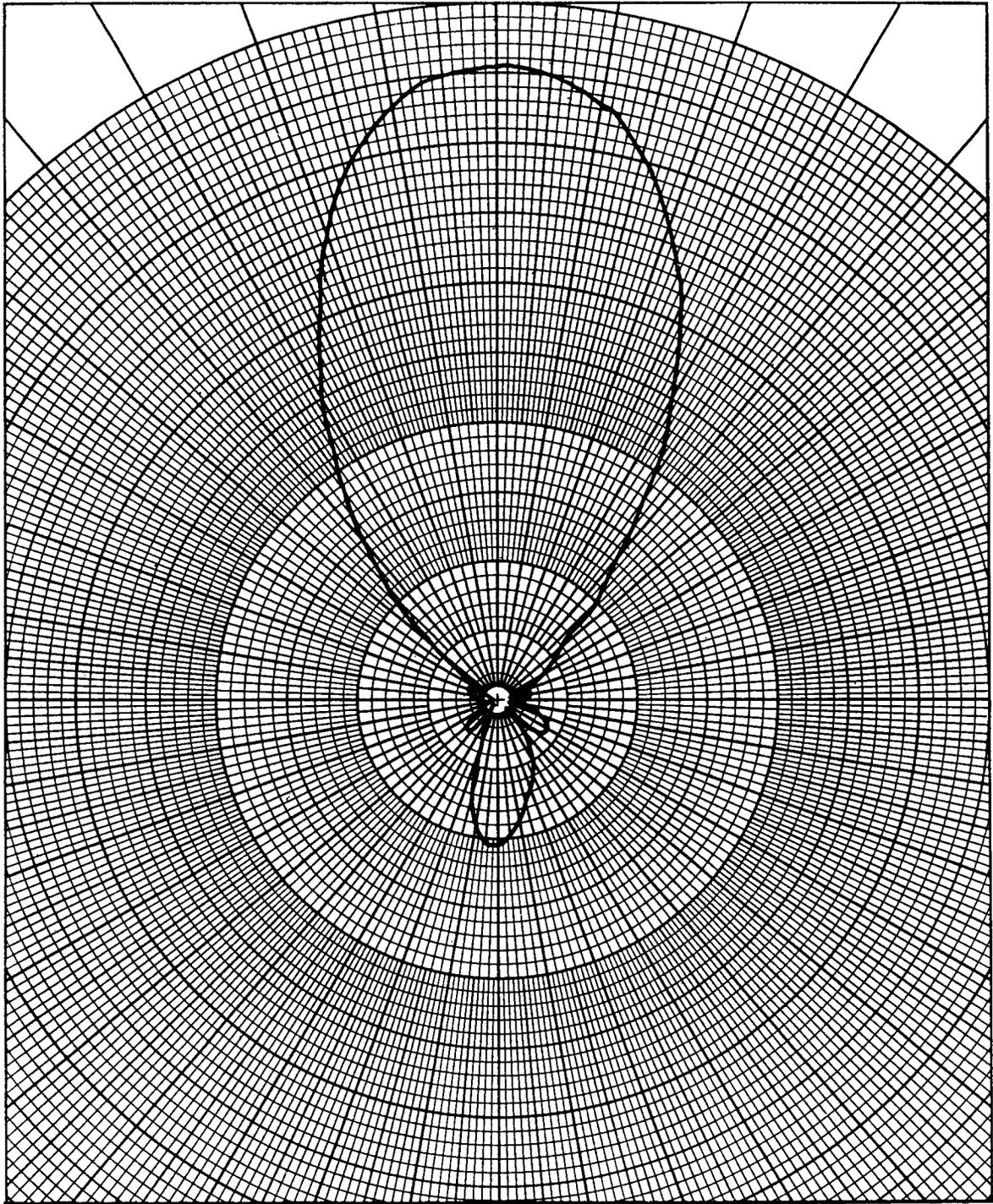
Figure 19. Radiation pattern in the E-plane of the five-element 0.8 wavelength long Yagi antenna (Deflection proportional to voltage)
