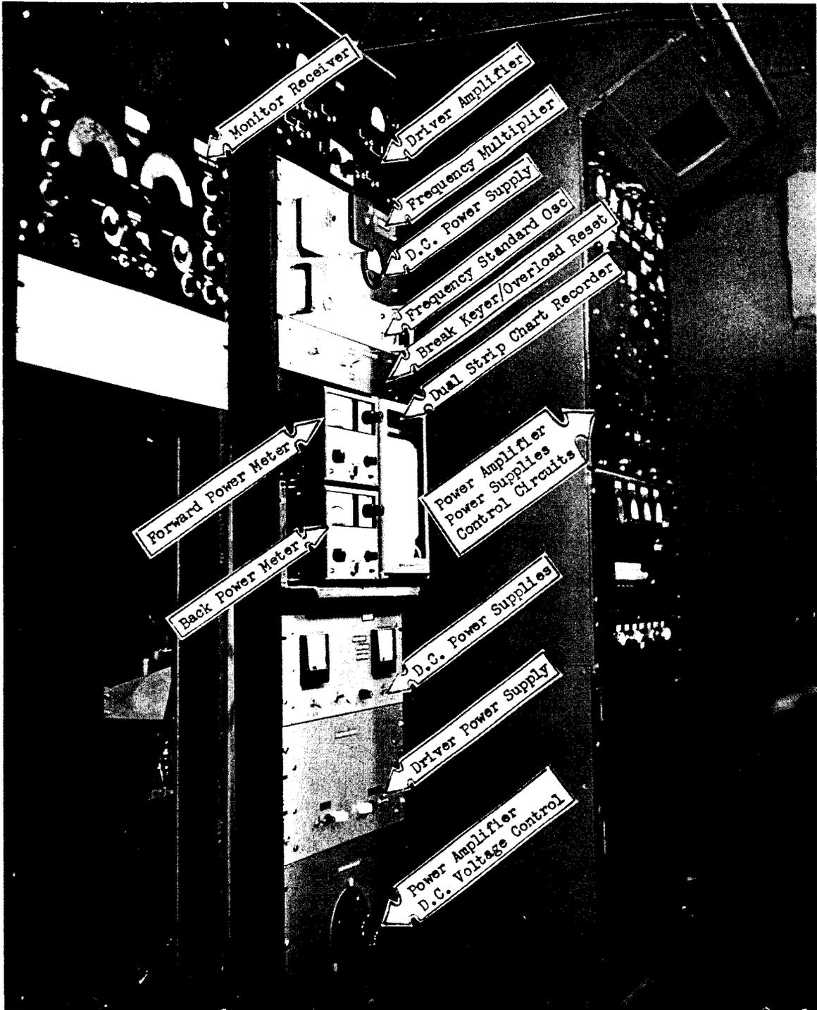
Figure 27. View of the power amplifier and associated control equipment
