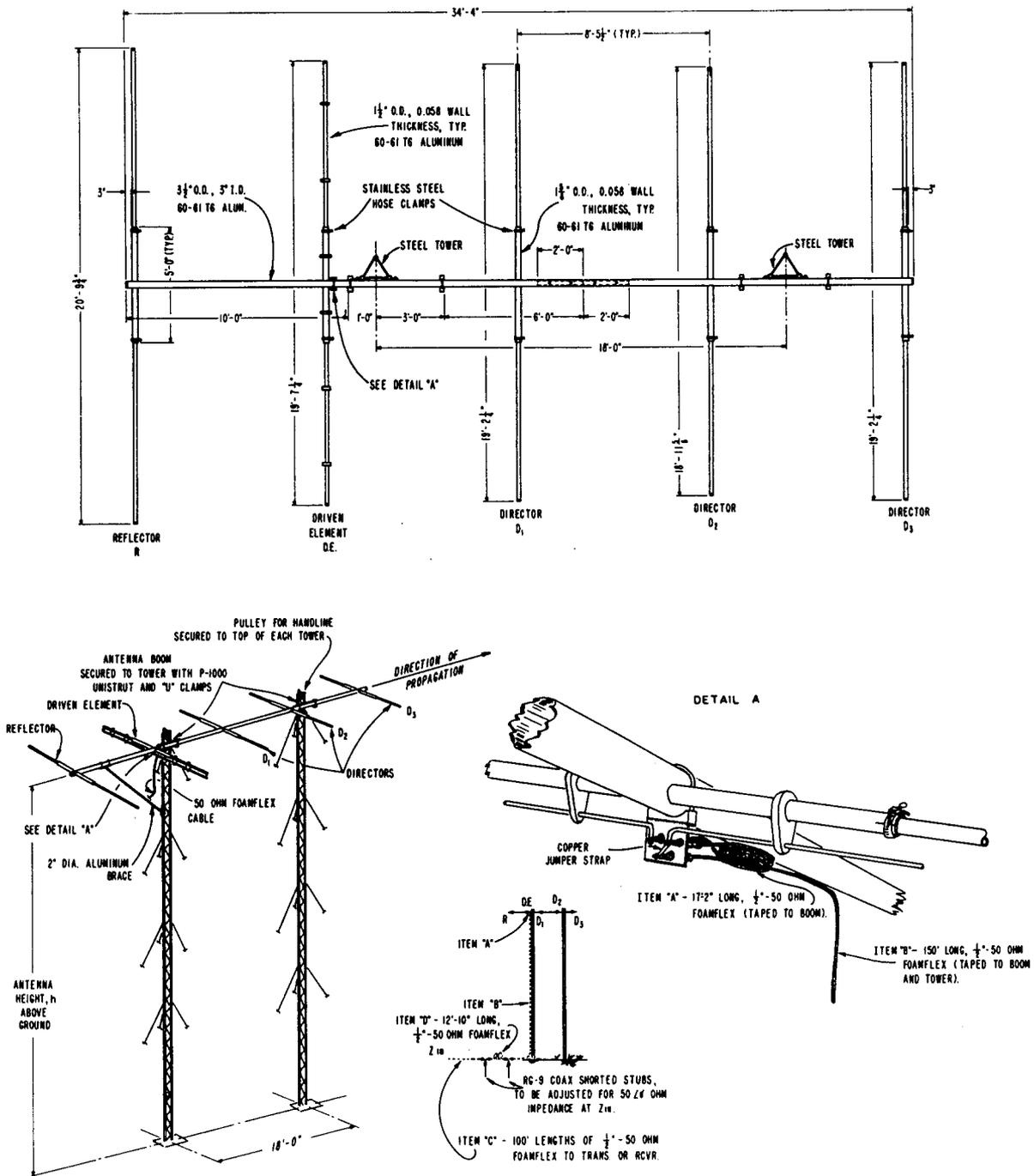
Figure 18. The 23 Mc/s five-element Yagi antenna design showing dimensions, mounting, and connection details
