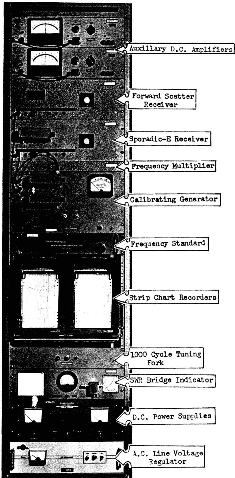
Figure 29. Photograph of the receiving equipment
