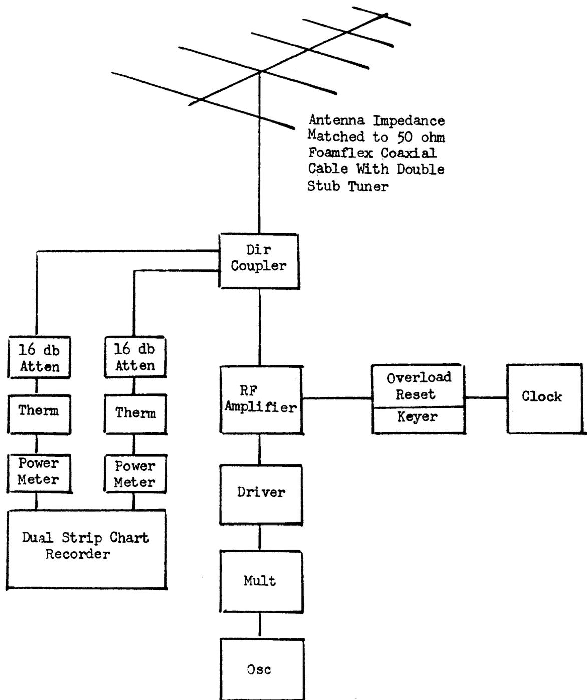
Figure 21. Block diagram of the transmitting system
