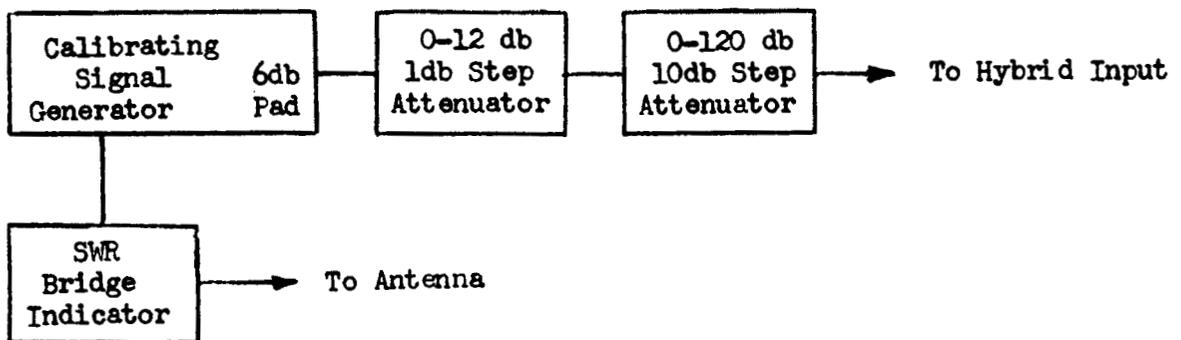
Figure 28. Block diagram of the receiving system
