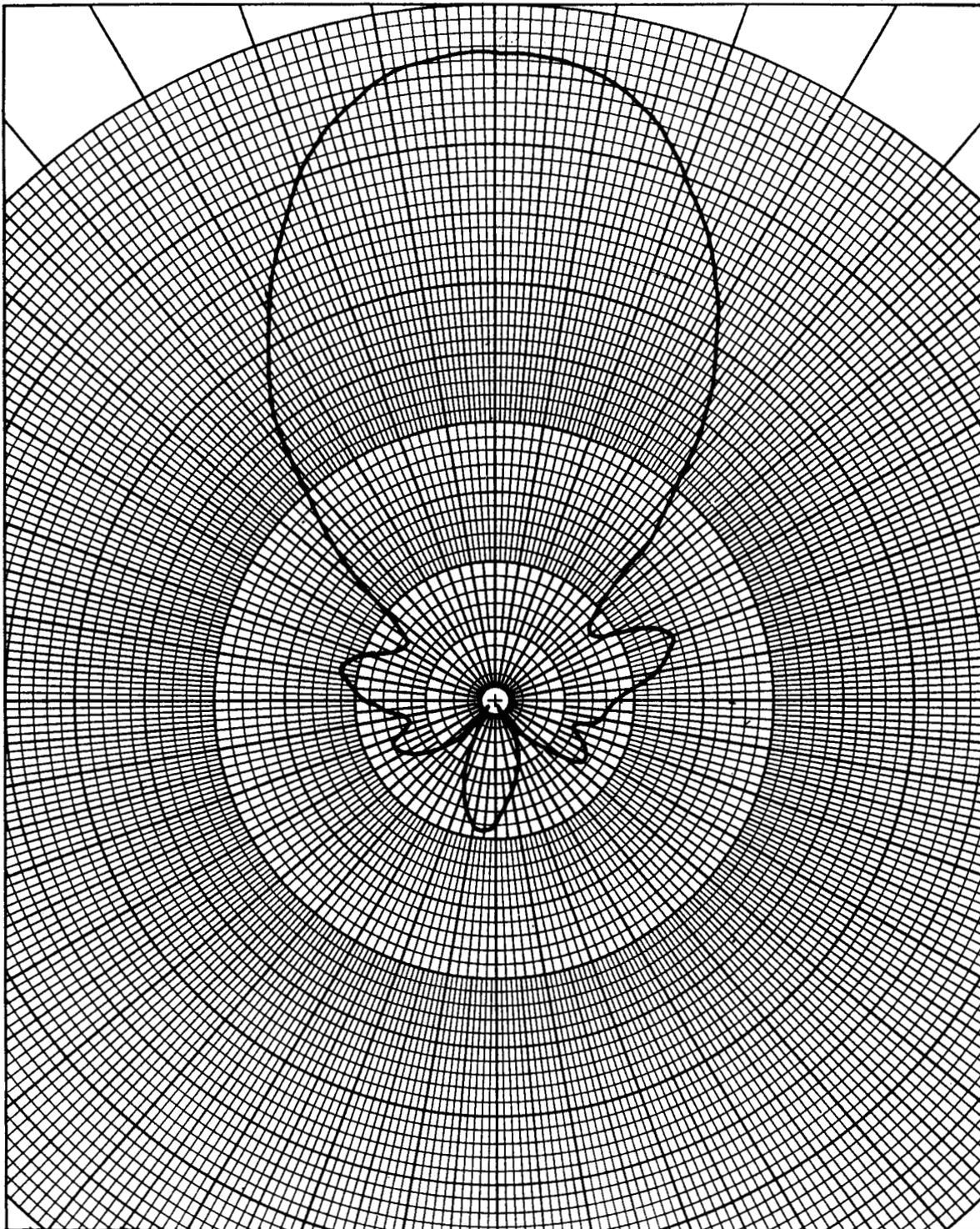
Figure 20. Radiation pattern in the H-plane of the five-element 0.8 wavelength long Yagi antenna (Deflection proportional to voltage)
