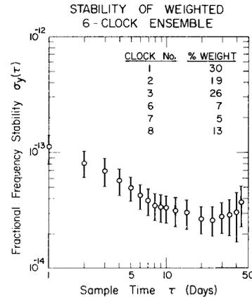
Fig. 1. Random noise fractional frequency stability of weighted 6-clock ensemble as determined from individual clock estimates. Clocks currently numbered 4 and 5 were not in the AT(NBS) clock ensemble at the time of this evaluation; however, the NP3 hydrogen maser was available and its signal was utilized during the evaluation [3]. This does not include any allowance for possible linear frequency drift of the ensemble.
