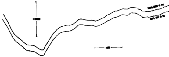
Fig. 5 A plot showing the detailed similarity of the time fluctuations of 60-Hz (power-line) clocks at NBS/Boulder, Colorado, and HP/Santa Clara, California. The 60-Hz clock at each site was compared with a local atomic clock.
