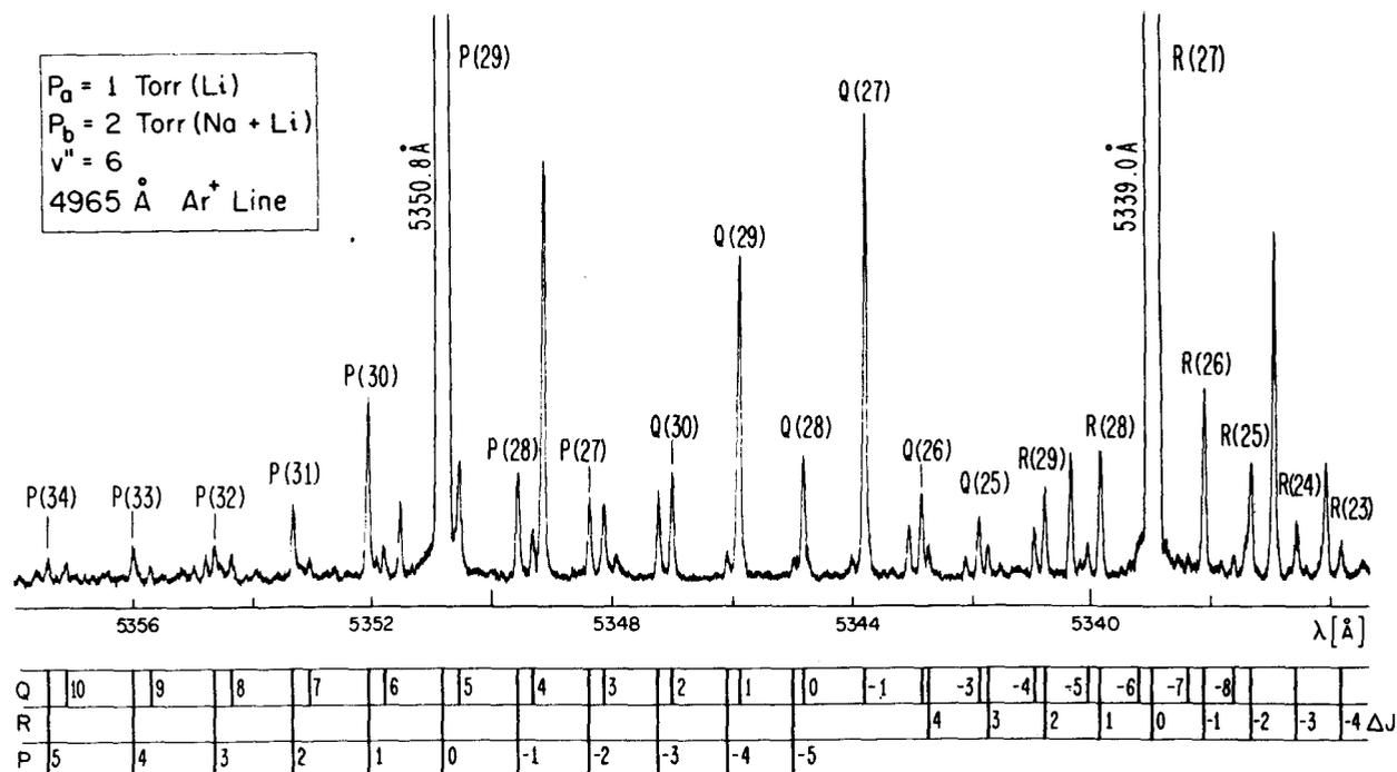
FIG. 4. Photoelectric scan of the NaLi resonance fluorescence spectrum generated by the 4965-Å line of the argon laser. The scan shows the member in the  $v''$  progression with  $v''=6$ . The changes of angular momentum  $\Delta J$  for the collision-induced satellite lines are marked below the scan.
