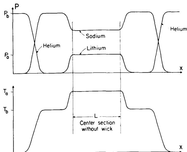
FIG. 3. Schematic diagram of the temperature distribution and of the partial pressures along the inside of the inner heat pipe.
