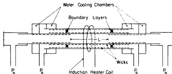
FIG. 2. Schematic diagram of the concentric heat-pipe oven which generates homogeneous arbitrary mixtures of a saturated vapor with an unsaturated vapor.
