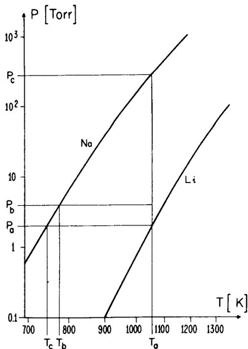
FIG. 1. Vapor pressure curves of sodium and lithium.
