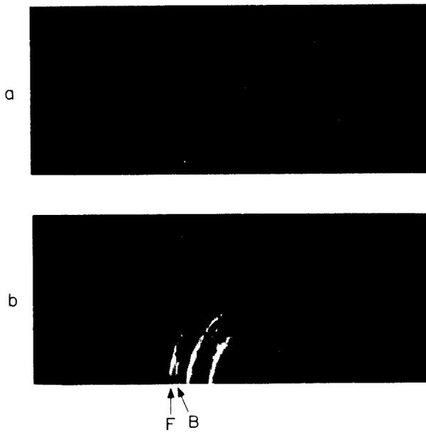
Fig. 3. Fabry-Perot fringes (a) of the *Q*-switched ruby laser radiation showing its single-frequency character and (b) of the off-axis Brillouin radiation showing *F*, the forward, and *B*, the backward component. In each interferogram the interorder spacing is  $0.50 \text{ cm}^{-1}$ .
