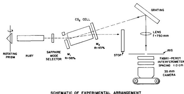
Fig. 1. Schematic diagram of the experimental arrangement.
