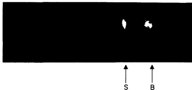
Fig. 2. Spectroscopic far field pattern of the output of the off-axis resonator, when the CS<sub>2</sub> cell was inserted in it. B, the stimulated Brillouin radiation; S, the first stimulated Stokes radiation.
