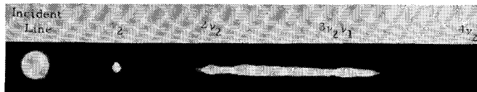
Fig. 2. Spectrum of the Raman laser output. The slit and the collimator are removed from the grating spectrometer, and the camera is focused at infinite distance.
