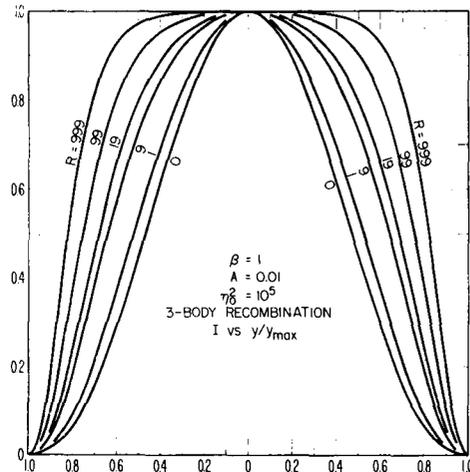
FIG. 3. Curves of relative luminous intensity as a function of radius within the tube for three-body recombination.
