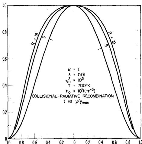
FIG. 2. Curves of relative luminous intensity as a function of radius within the tube for collisional-radiative recombination at 700°K.
