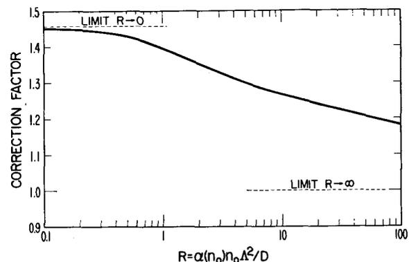
FIG. 4. Value of the factor,  $1/\int \Phi d(y/y_{\max})$ , as a function of the ratio  $R$ , of recombination loss rate to diffusion loss rate at the center of the plasma.
