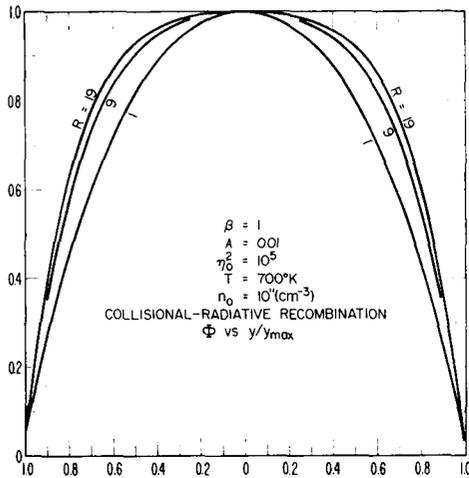
FIG. 1. Curves of relative electron density as a function of radius within the tube for collisional-radiative recombination at 700°K.
