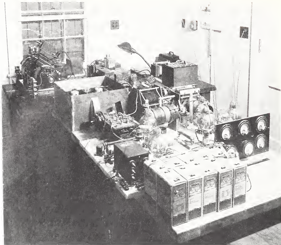
Radio transmitter (front) and receiver with recorder (rear) for automatic recording of virtual heights of ionosphere. This first automatic multifrequency recorder (or ionosonde), with a frequency range of 2500 to 4400 kHz, was developed by Gilliland in 1932 and installed in Building No. 3 at the Beltsville, Md. field station, and later moved to the Meadows, Md. field station.
