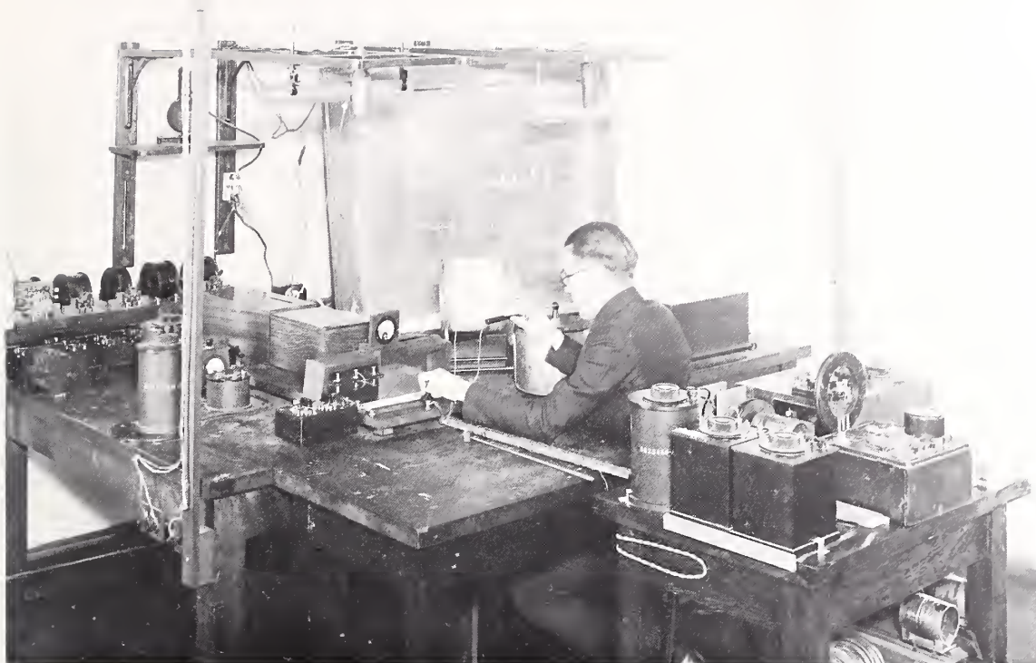
A balanced-transformer method for the rapid measurement of capacitance, inductance, and resistance at radio frequencies, described in a 1924 Bureau publication by August Hund. Later, Hund authored several well-known technical books on radio subjects.
