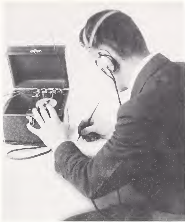
Receiving market reports to monitor the Bureau's station, WWV, during the winter of 1920-1921. The experimental program was initiated at the request of the Bureau of Markets, Department of Agriculture, using a 2-kW spark transmitter and code. Reception in this photograph was on a commercially produced crystal set.
