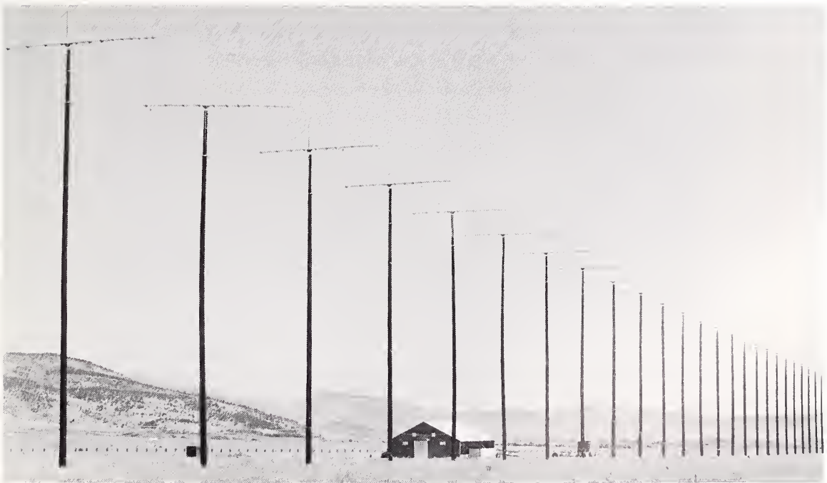
Combination (upper left) of two electronically-scanned antenna arrays of high resolution for simultaneous horizontal and vertical scanning to study the ionosphere in the frequency range of 12 to 25 MHz, including the effects of ionospheric irregularities on radio-signal propagation over long distances. The array for horizontal scanning (lower photo) consists of 25 masts, each mounted with a log-periodic dipole antenna of 13 elements. In the close-up skyward view (upper right) can be seen 8 of the 10 log-periodic dipole antennas (13 elements) for vertical scanning, mounted at 16-meter intervals on the 152-meter tower. This combination of two antenna arrays is one of many specialized facilities located at the Table Mountain field station, beginning in 1954.
