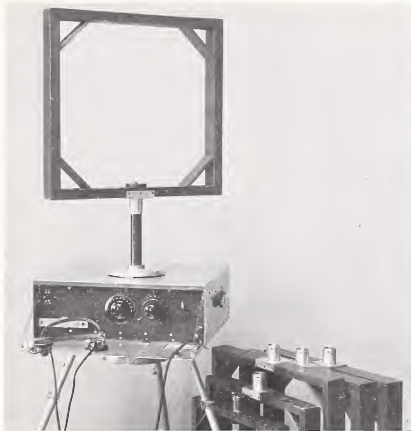
A portable-type direction finder developed by Dunmore in 1925 for the Navy and the Army Signal Corps. It was known as a "universal" type because of the wide frequency range—90 to 7700 kHz, using seven sizes of loop antennas. A single tuning control was one of the many features.
