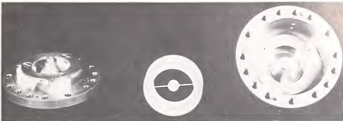
Quartz ring or toroid crystal unit used in Section II of the National Primary Standard of Radio Frequency as a further development in quartz crystal technology. The 200-kHz quartz crystal ring (center) is supported by two arms which are part of the mother crystal. Sections of crystal housing are shown at left and right.
