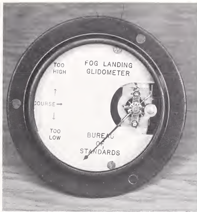
Early form of landing beam indicator. Used by pilot to follow proper glide angle in a blind landing.
