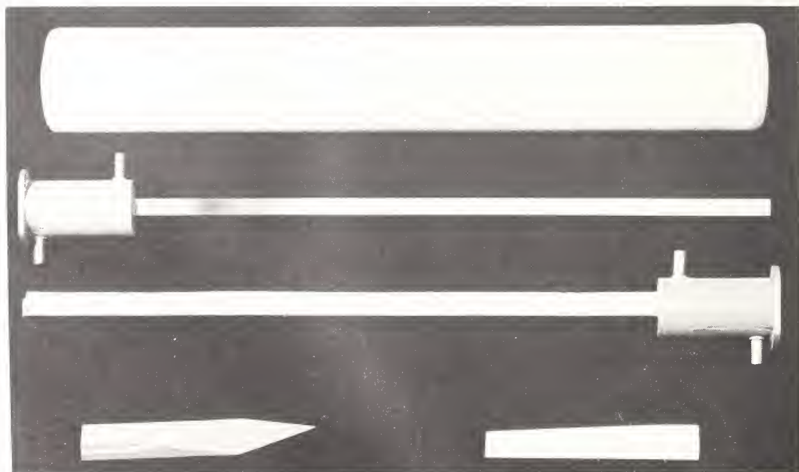
By 1962 a microwave noise source operating at more than 1000 °C, suitable as a reference standard, was achieved. One combination of elements was a silicon carbide load resistor termination (lower left) with a gold waveguide (lower center). Another combination was a zinc titanate load with a platinum-rhodium alloy waveguide (upper center). Each was contained within a graphite heat distributor, coated with zirconium dioxide (upper).
