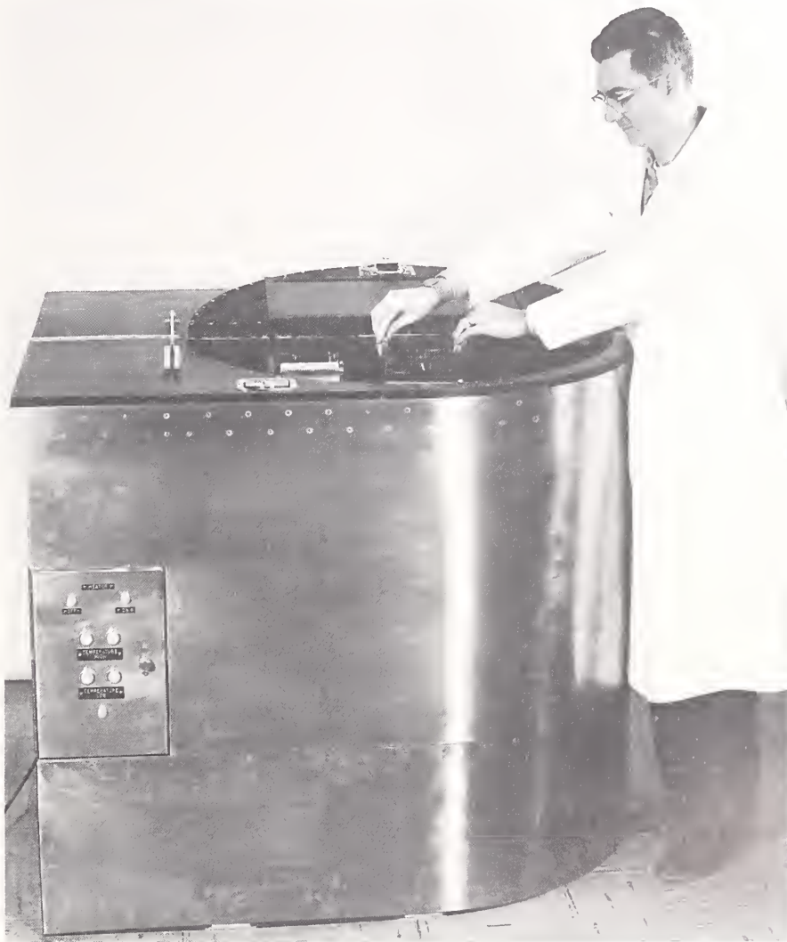
Controlled-temperature oil bath, for saturated standard cells, developed in 1960 by Patrick Lowrie (in photo) of the Electronic Calibration Center. This bath of advanced design combined many novel features for temperature control, ease of handling and circulating the nearly 100 gallons of mineral oil, and easy means of inserting and removing standard cells. Two baths were constructed, one for operation at 28^\circ\text{C} , the other at 35^\circ\text{C} . Control of oil temperature was within \pm 0.002^\circ\text{C} per day. In 1966 the two baths were transferred to the Electricity Division at NBS Gaithersburg.
