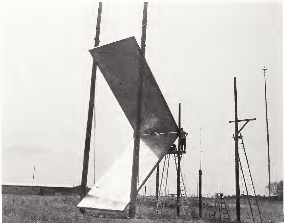
Large corner-reflector antenna erected at the Sterling field station for study of antennas suitable for communication by ionospheric forward scatter. The sheet-aluminum reflector surfaces could be set at various aperture angles, shown in the photo of October 1953 at 90°. Barely distinguishable near the vertex is the single half-wave dipole radiator (for operation at 400-MHz measurement frequency) at one of the two positions. Measurements of antenna gain were made as a function of aperture angle and different widths and lengths of reflector surfaces (in terms of wavelengths). Photo shows reflector size of 25 ft length and 12 1/2 ft width (across vertex).
