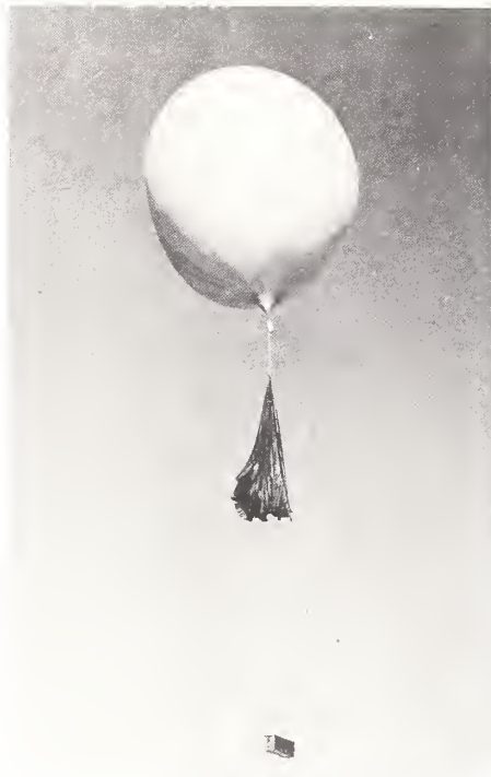
Balloon-borne pulse repeater, attached to parachute, for determination of wind velocity to altitudes of 60,000 ft by radar method. Parachute provided for slow descent of 3-lb repeater after bursting of balloon at high altitude.
