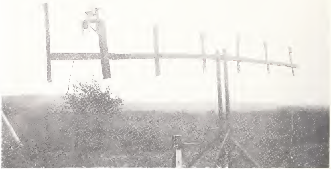
Earliest form of directive antenna array at College Park Airfield for glide-angle or landing beam for blind landing of aircraft. A 93.7-MHz transmitting oscillator fed the radiating dipole antennas. Other horizontal antennas served to direct the narrow landing beam.
