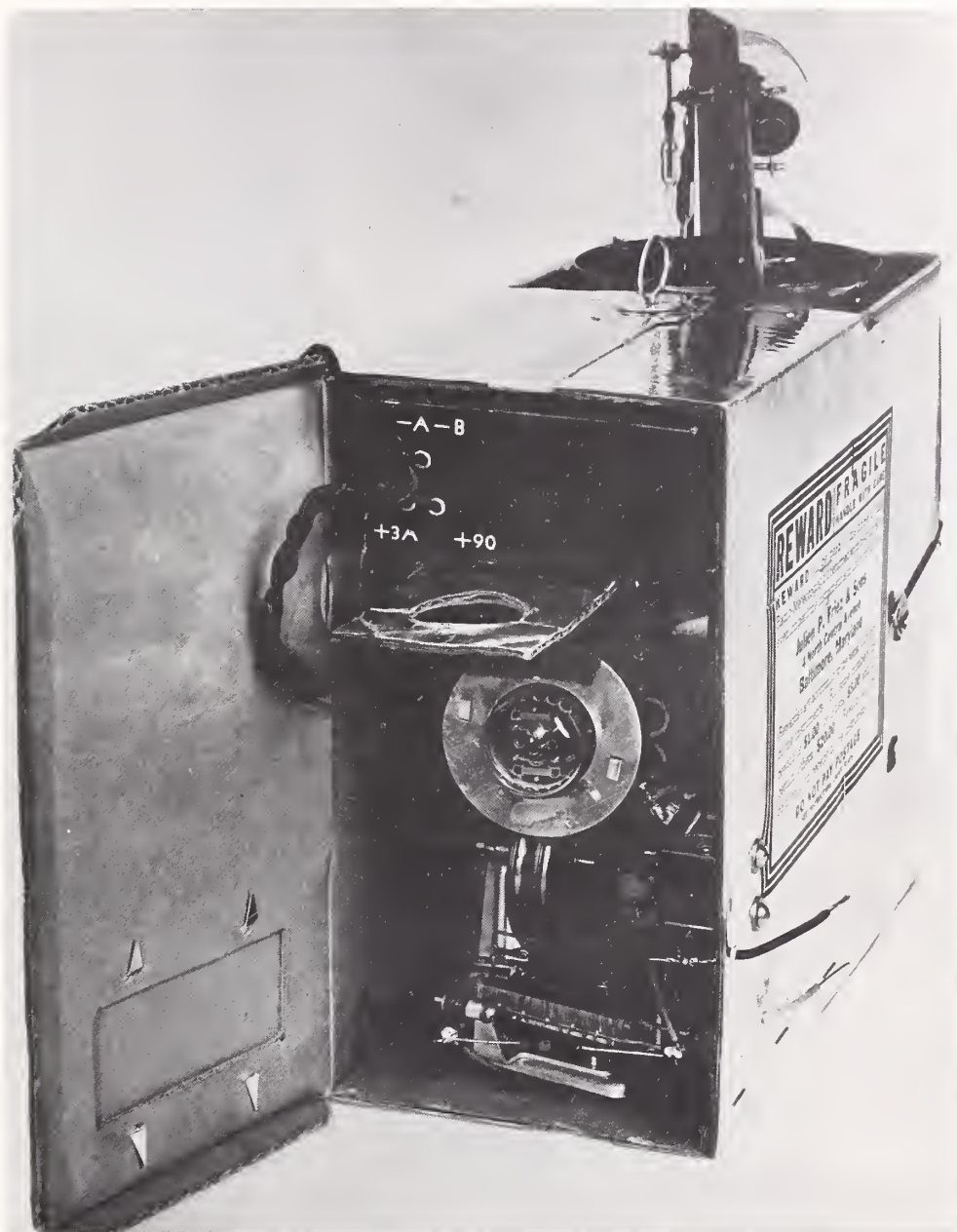
This radiosonde was manufactured in large quantities by 1940, and incorporated improvements developed by the Radio Section. The batteries, transmitter, and pressure unit were housed in an insulated box to minimize temperature changes. Temperature tube and electric hygrometer (at rear) were shielded against solar radiation by double-walled metal tube. Total weight less than 1 kg; cost was $25 in 1940. The finder, after balloon flight, received a monetary award upon return of radiosonde to Bureau.
