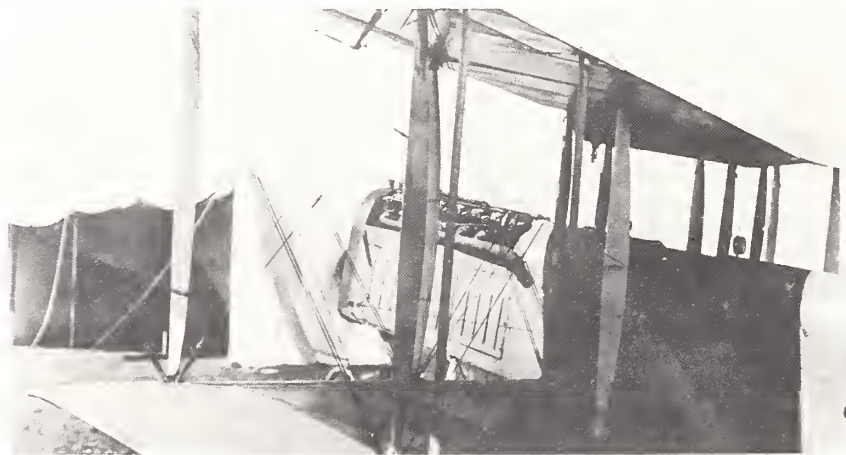
Post Office Department biplane used by Radio Section at College Park, Md. Airfield in early 1919 for landing experiments. Two coils, one under each lower wing, could pick up the low frequency (500 Hz) induction field from a large coil encircling the field, with the plane at several thousand feet altitude. A tent in the background served as a temporary hanger.
