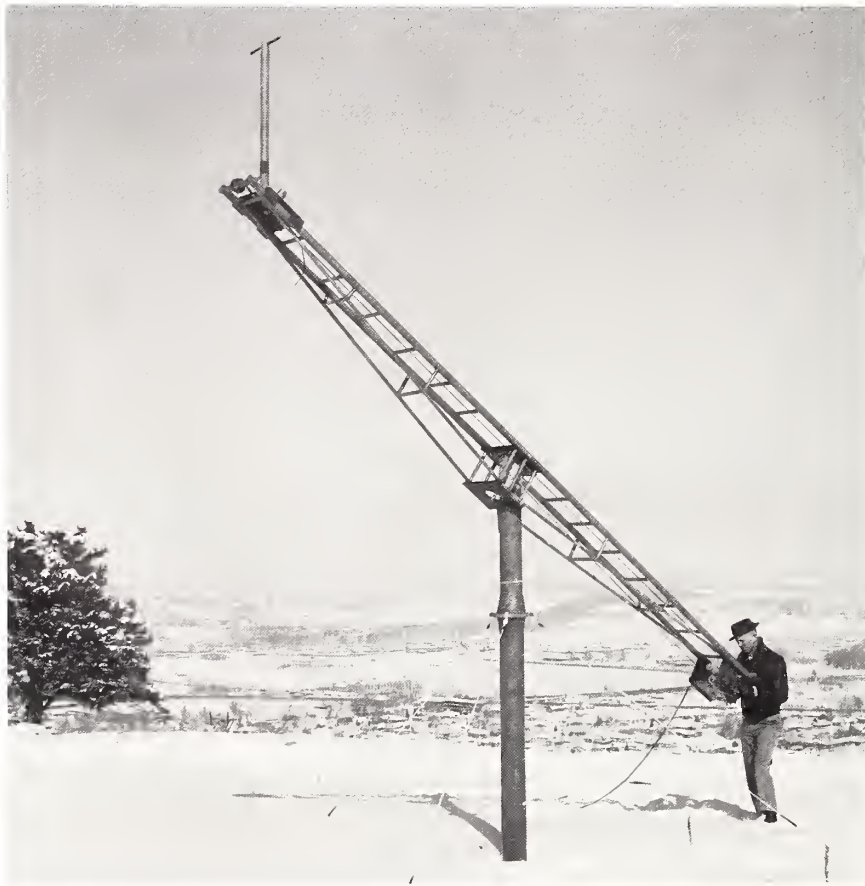
Carriage-and-track mounting designed by the Antenna Research Section for positioning a dipole antenna in three mutually perpendicular directions along three orthogonal axes, with the measurements related to those of a second dipole in a fixed position (not shown). Subsequent computer processing of the measurements yields the amplitude, phase, and angles of arrival of the multipath field components in this aperture-synthesis method. Photo shows the experimental system located at the Bureau's elevated site on Green Mountain Mesa, with a view to the northeast overlooking Boulder.
