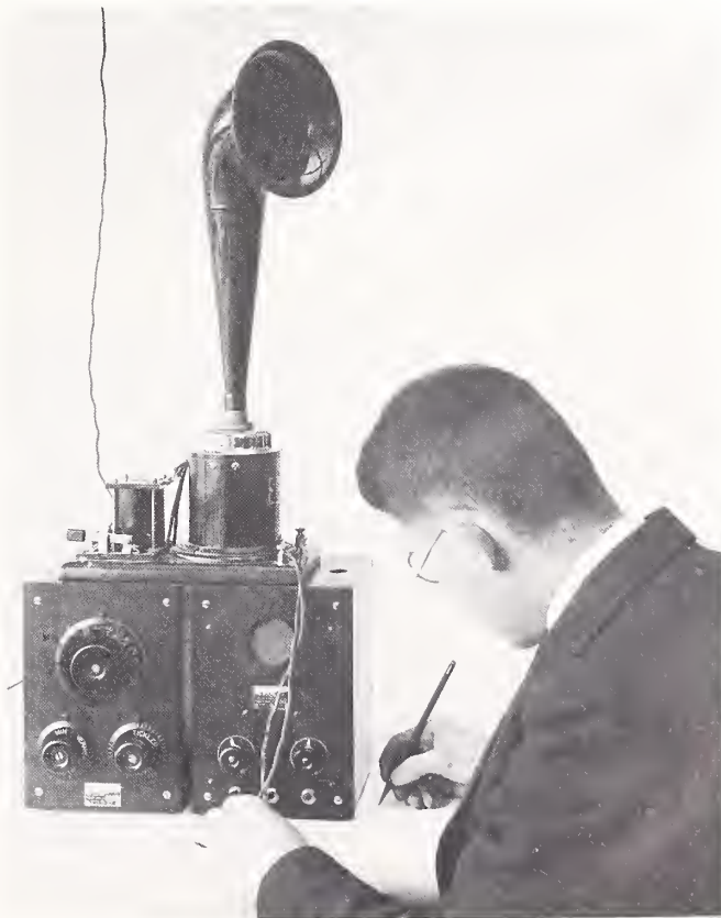
Receiving market reports in code with a very early commercially produced three-tube regenerative receiver designed for broadcast reception. The loudspeaker was an early design that had considerable popularity during the first years of broadcasting.
