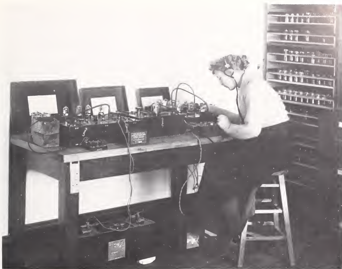
Laboratory equipment for measuring the characteristics of electron tubes for use as detectors, amplifiers, and oscillators. Due to lack of performance information by manufacturers of tubes, the Radio Section, at the request of the Army Signal Corps, initiated a measurement program during World War I that was continued until 1924 when such information became readily available.
