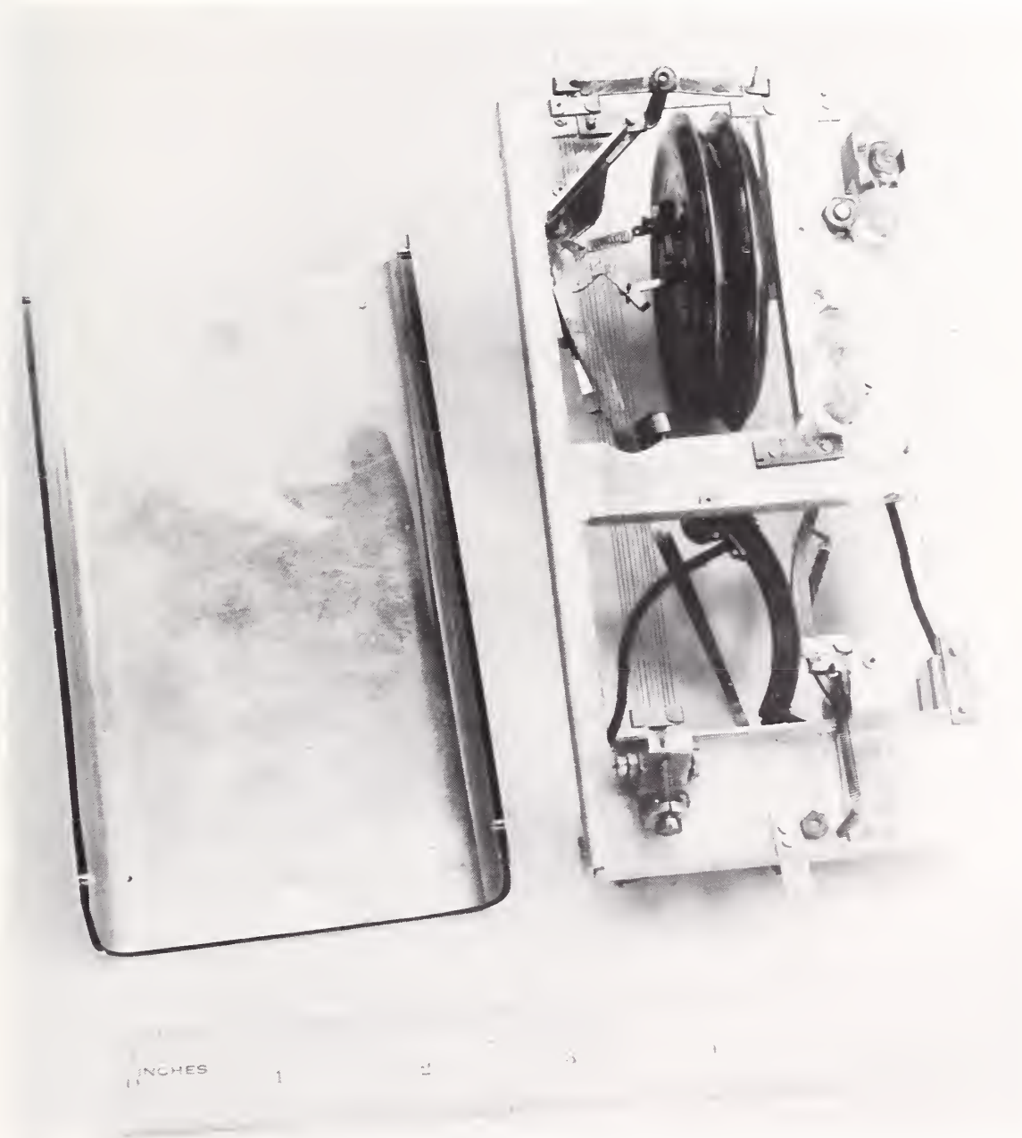
The earliest model (1936) of radiosonde constructed for Radio Section by a commercial firm on a Navy Project. At upper right is one type of electrolytic resistor (in glass tubing) used as the temperature sensor. The two sections of hair hygrometer for measuring relative humidity are clearly shown, as well as a side view of the aneroid barometer. Electron-tube circuitry forms another portion of the chassis.
