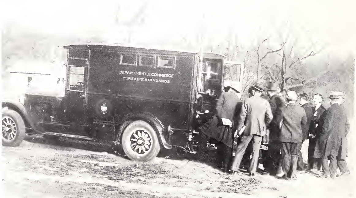
Delegates to International Radio Conference, Washington, D.C. in fall of 1927, inspecting the mobile radio laboratory at the Bureau of Standards. The laboratory truck was used in various parts of the country to make field measurements of fading and intensity of radio signals.
