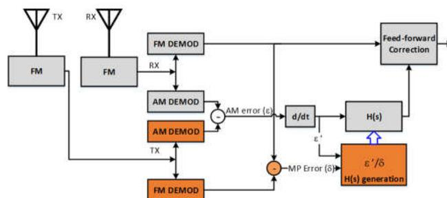
Fig. 1. Block diagram of the FM-AM correlation measurement and compensation technique. The orange blocks are required only for H(s) generation. H(s) is the control transfer function that maps amplitude fluctuations to multipath (MP) error. In case of two-way ranging known modulation symbols can be used for H(s) generation.
