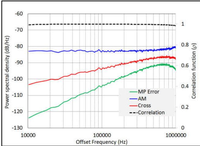
Fig. 2. Plot of the power spectral density  $S_{\delta\varepsilon}$  (cross) along with  $S_\delta$  (multipath error) and  $S_\varepsilon$  (AM) (left axis). The plot shows almost 100 % correlation ( $\rho = 1$ ) as shown on the right axis. For this simulation, a 100 MHz carrier frequency modulated with white noise (standard deviation = 0.1, noise bandwidth = 1.0 MHz, modulation index = 0.3) and multipath delay,  $\tau = 13$  ns was used. MP – Multipath.
