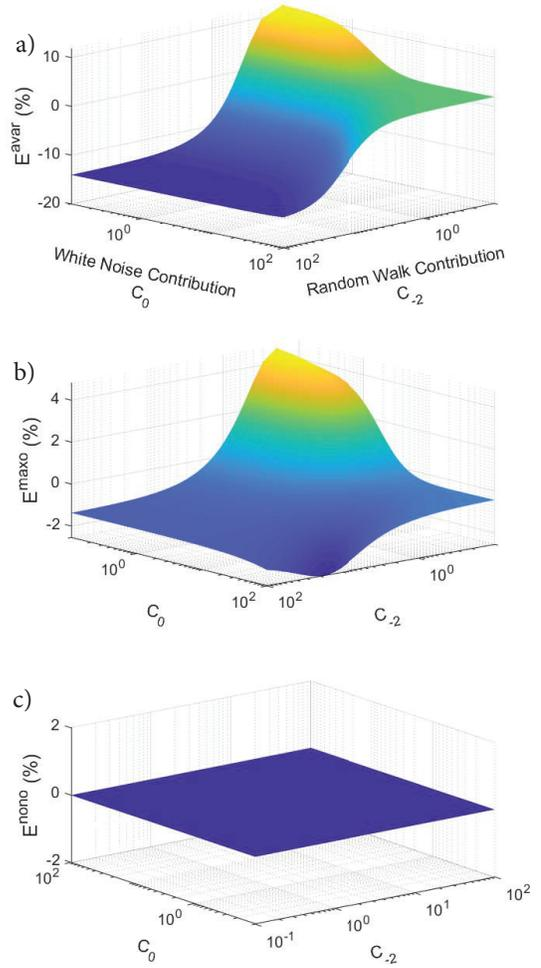
Fig. 1. The error in the estimation of SVAR by the sums over powers of two of (a) the Allan variance, (b) the maximally overlapping Allan variance, and (c) the non-overlapping Allan variance as functions of the ratio of white noise  $C_0$  and random walk noise  $C_{-2}$  to flicker. Simulated power law noise samples were obtained from Neil Ashby and were generated using the techniques outlined in [7].
