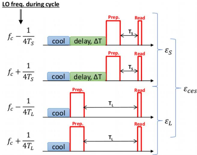
**FIG. 2.** The experimental sequence for CES spectroscopy with a cold-atom CPT clock. Two sub-sequences, each composed of two Ramsey-interrogations, are applied. Each interrogation begins with a cooling period. For clock interrogations with a short dark period  $T_S$ , a delay of  $\Delta T = T_L - T_S$  is introduced between the end of the cooling phase and the beginning of the Ramsey interrogation.
