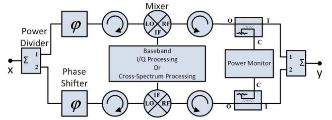
Fig. 7. Block diagram of the two-channel  $W$ -band standoff vibrometer. The signal input to ports “x” and “y” is the same as that of Fig. 1.
