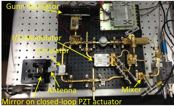
Fig. 2. Experimental realization of the single-channel W-band stand-off vibrometer. Here, the target is a mirror on closed-loop PZT actuator. A W-band Gunn oscillator with DSB noise,  $S_{\phi-\text{Gunn}}(f) = +77 f^{-3}$  dBrad<sup>2</sup>/Hz at 95 GHz is used as the reference carrier and a feedhorn antenna with 20-dB gain is used.
