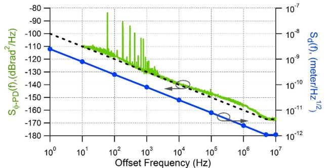
Fig. 5. Plot of the DSB phase noise of the PD at 95 GHz and the corresponding PSD of the displacement.
