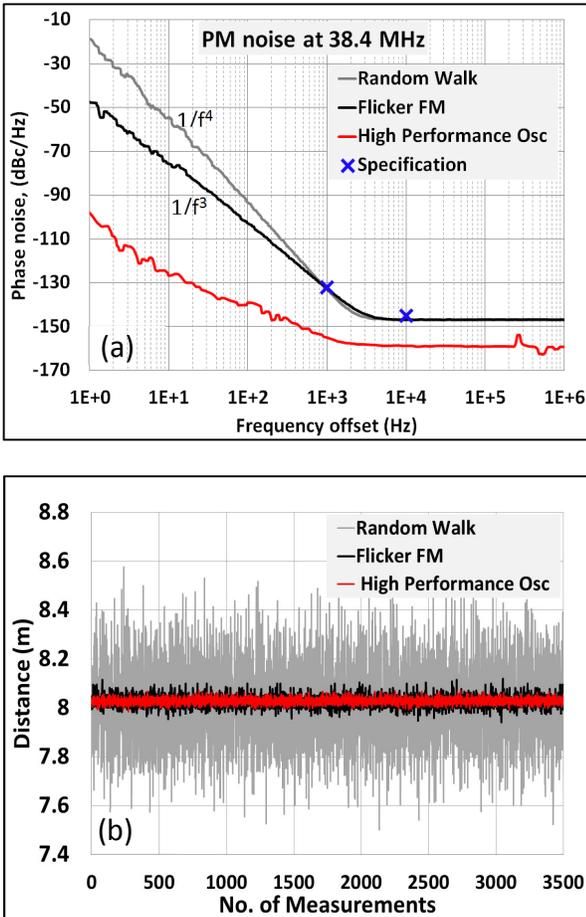
Fig. 2: (a) Three different phase noise levels of the local oscillator at 38.4 MHz (b) corresponding distance measurement.
