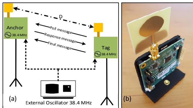
Fig. 1: Two-way ranging scheme used by the DUT. The range is calculated from the time-of-flight obtained from the receive and transmit time stamps of three messages. The DUT was evaluated with internal as well as external 38.4 MHz local oscillators. (b) Picture of one of the transceiver.
