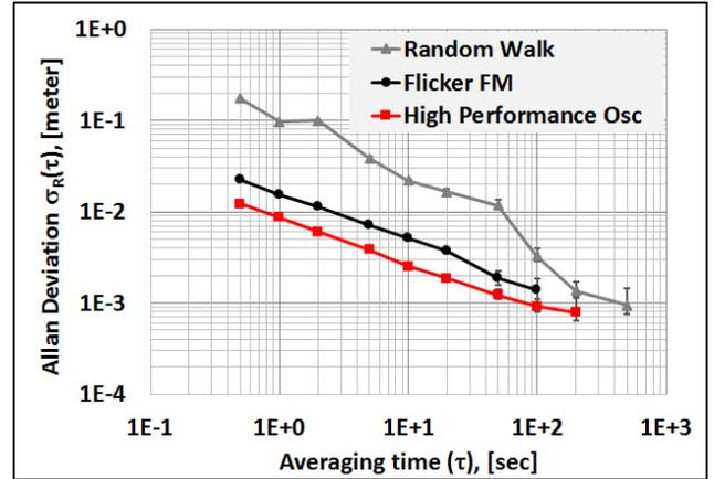
Fig. 3: Plot of ranging stability  $\sigma_R$  obtained from ADEV for different phase noise values of the local oscillator.
