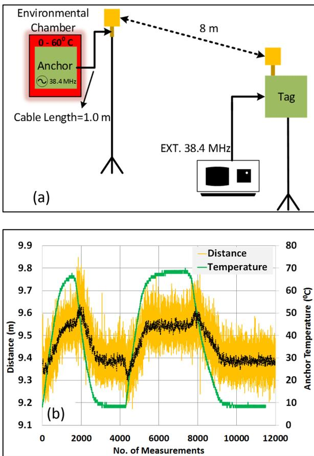
Fig. 4: (a) Mounting of the anchor inside the environmental chamber. (b) Effect of frequency drift of the LO due to temperature on the distance measurement. The black dotted curve is obtained from 20 moving averages.
