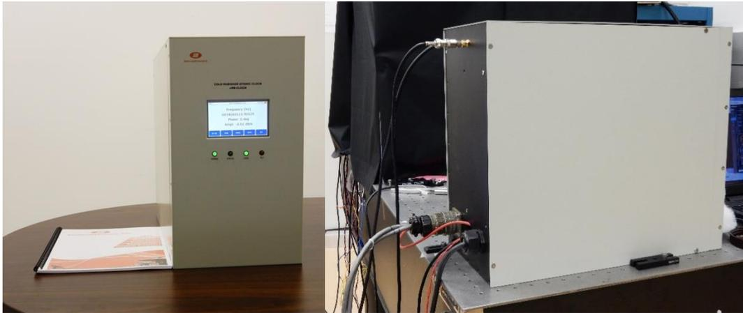
**Figure 1** – Prototype of the portable cold  $^{87}\text{Rb}$  atomic clock. The clock is packaged in a 22 x 37 x 32 cm enclosure and weighs about 28 kg. The signal and power connections are on the rear panel of the instrument.
