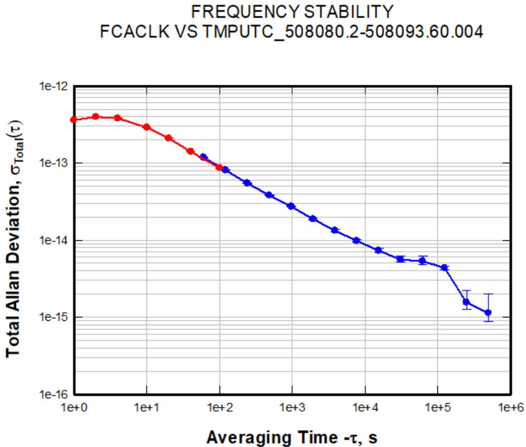
**Figure 2** – Total Allan Deviation of the cold Rb clock as measured against UTC(NIST). No drift has been removed. The 1 s data is shown in Red, while the 60 s data is shown in Blue. The noise between ½ and 2 days is under investigation.
