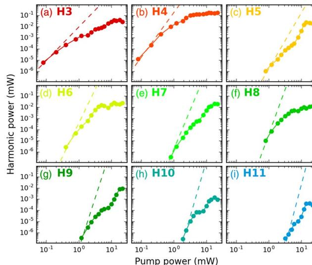
**Fig. 4.** Integrated power of each harmonic order as a function of the pump power. At lower powers, the harmonics show a perturbative behavior, scaling roughly with  $p^n$  (dashed lines), where  $p$  is the pump power and  $n$  is the harmonic order. At higher powers, a non-perturbative scaling is observed. For H9, H10, and H11, a step is seen at approximately 10 mW, which corresponds to the situation where the discrete harmonics spectrally broaden and begin to merge together.
