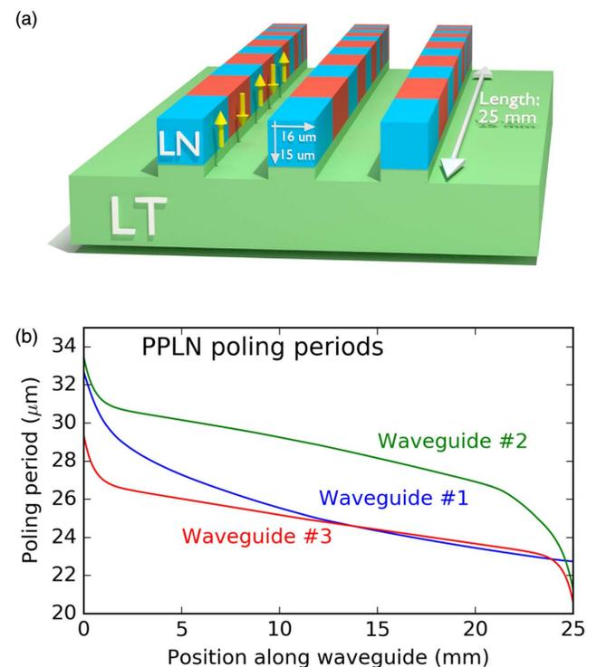
**Fig. 2.** (a) An illustration of the chip containing the lithium niobate (LN) waveguides on a lithium tantalate (LT) substrate. The pitch of the domain inversion periodic poling (shown as red and blue regions) changes along the length of the waveguide. The poling period is exaggerated for clarity; the waveguides contain several hundred poling periods. (b) Each waveguide has a different rate of chirp for the poling period.
