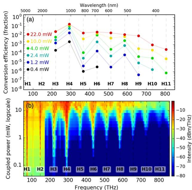
**Fig. 3.** Conversion efficiency of the harmonics (a) and the output spectrum (b) at various pump power levels. For these results, Waveguide #2 was pumped in the increasing-poling-period direction. (Note: Below 170 THz, the spectra were collected using a mid-infrared optical spectrum analyzer, which has a higher noise-floor.)
