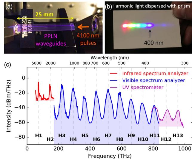
**Fig. 1.** (a) When pumped with mid-infrared light, the periodically poled lithium niobate (PPLN) waveguide glows with visible light. (b) The generated light, as dispersed with a prism and observed on white paper, reveals harmonic peaks across the visible and ultraviolet regions. (c) When pumped with 20-nJ,  $\sim 200$  fs pulses of 4100-nm light, the output spectrum consists of harmonics up to the 13th order (H13 at 315 nm).
