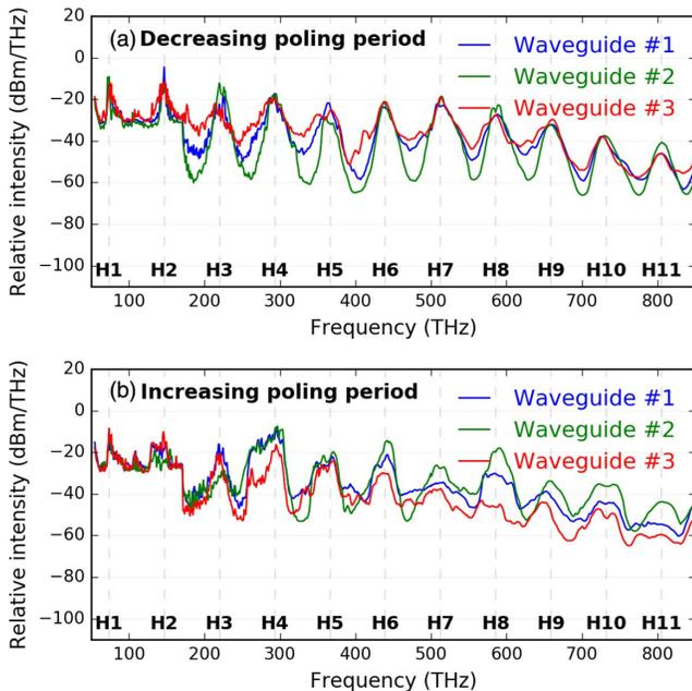
**Fig. 6.** PPLN waveguides pumped with 25-nJ pulses exhibit broader harmonic peaks. (a) When pumped in the decreasing-poling-period direction, small differences are seen between the various waveguides, mainly in the regions between the harmonic peaks. (b) When pumped in the increasing-poling-period direction, large differences are seen in the spectra produced from the various waveguides.
