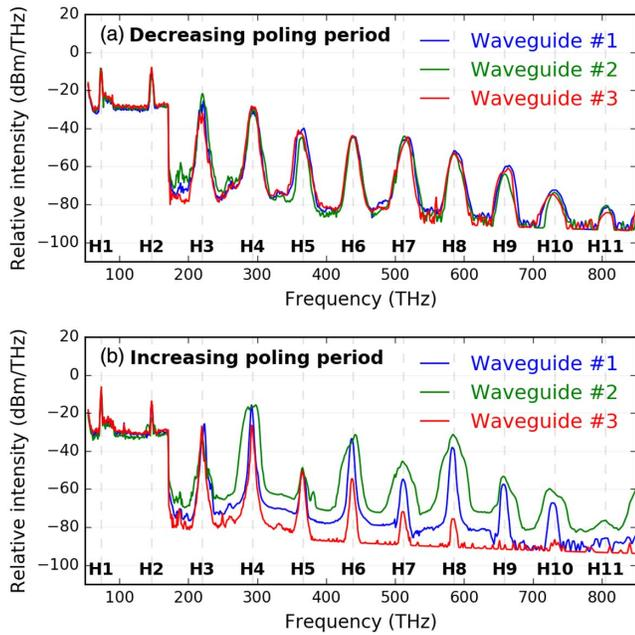
**Fig. 5.** PPLN waveguides pumped with 5-nJ pulses. (a) When pumped in the decreasing-poling-period direction, a smooth spectrum of even and odd harmonics is seen, with minimal changes between the waveguides. (b) When pumped in the increasing-poling-period direction, significant differences are seen between the different waveguides.
