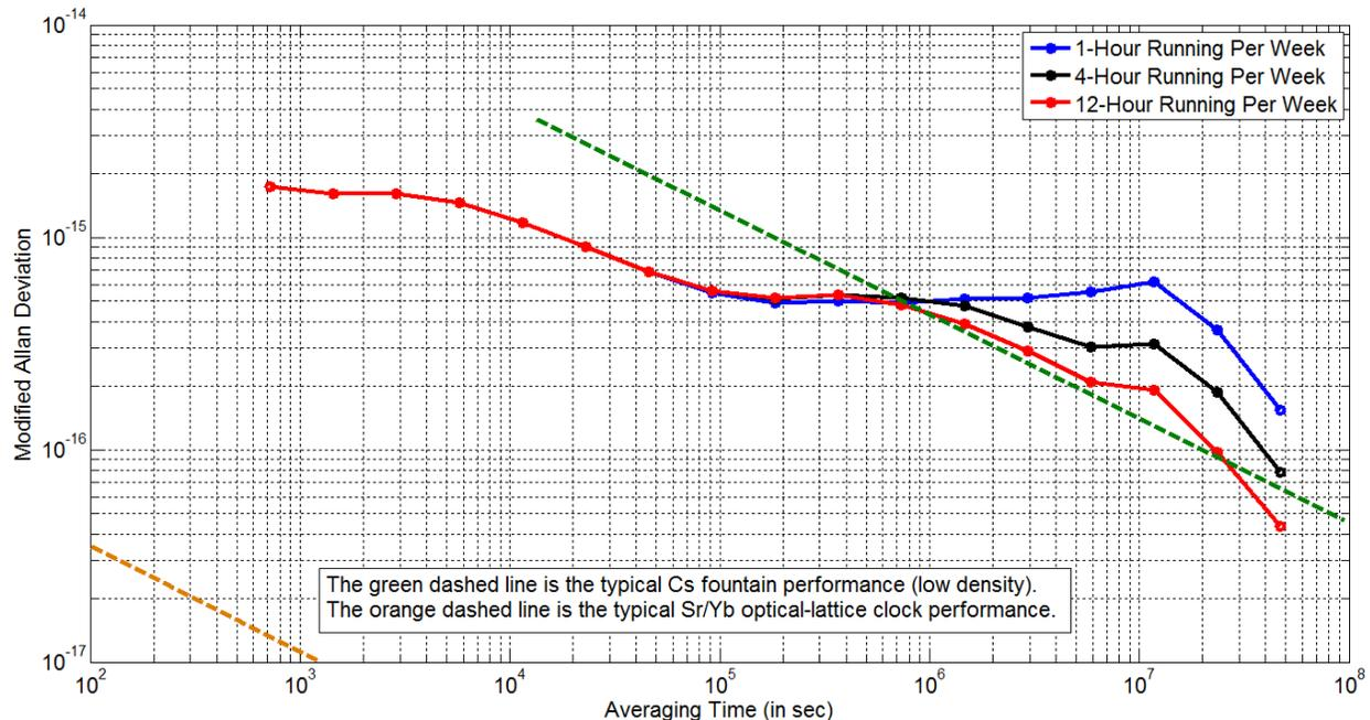
Fig. 7. Running an optical clock once a week.
