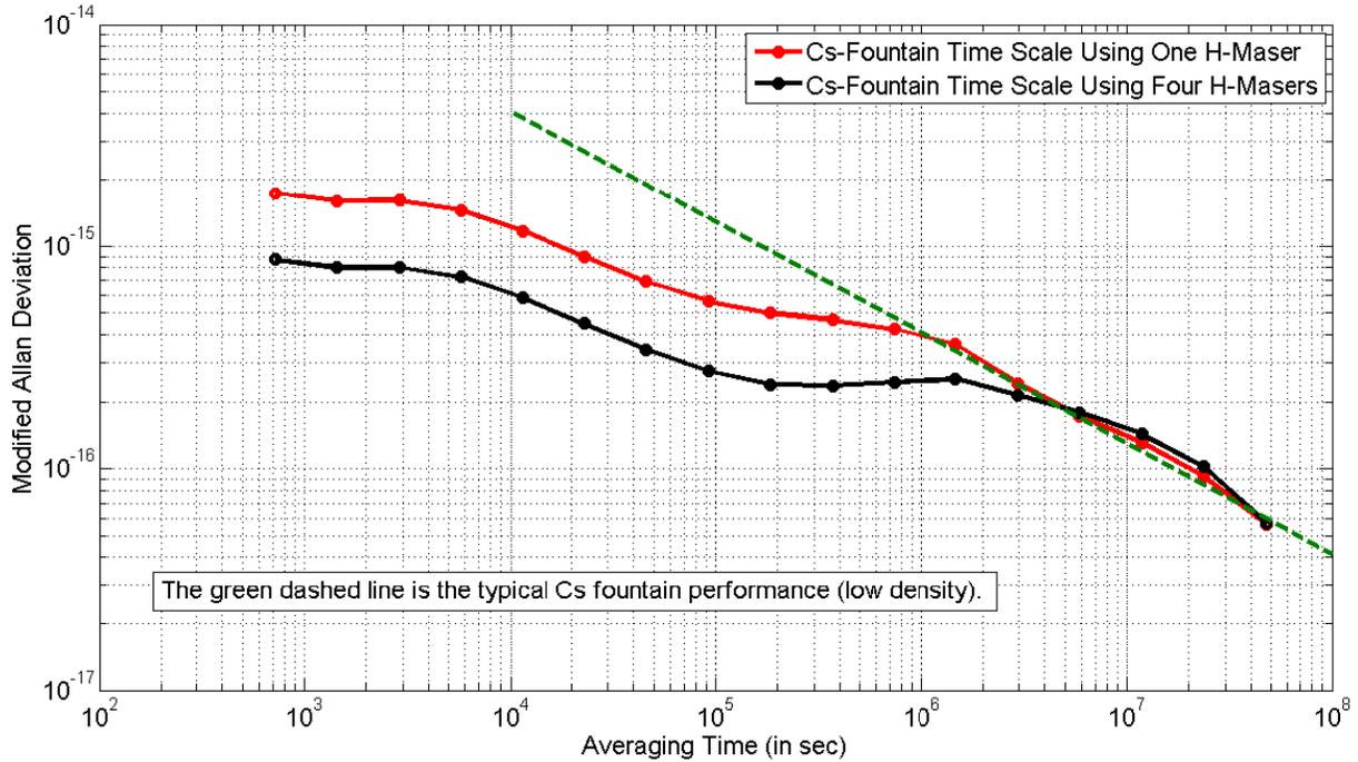
Fig. 3. Performance of a time scale steered to a continuously operating cesium fountain. The green dashed line shows the performance of the cesium fountain. The solid curves show the stability of a steered time scale that contains one or four masers.
