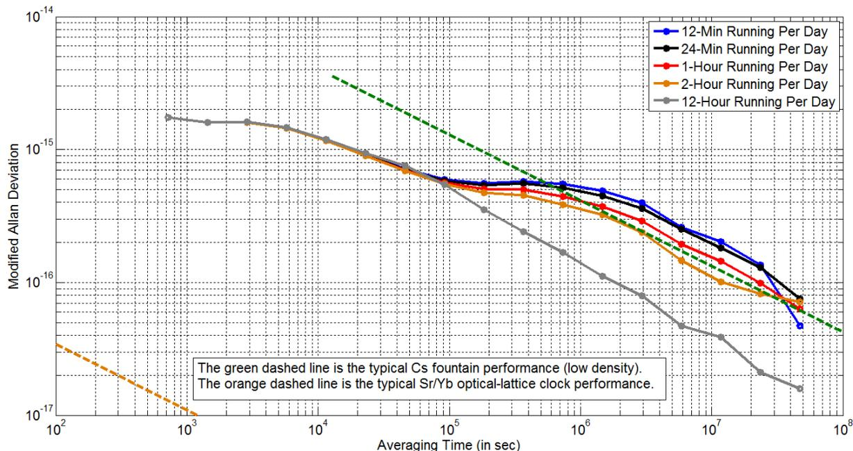
Fig. 5. Running an optical clock once a day.
