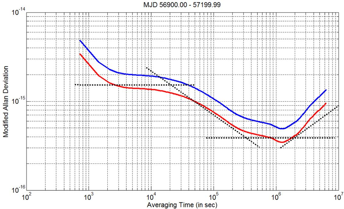
Fig. 1. The blue curve shows the frequency stability of the time difference between two NIST H-masers. The red curve shows the estimated frequency stability of a single H-maser, assuming that the two masers have the same statistical characteristics. We model the stability as shown by the black dotted lines.
