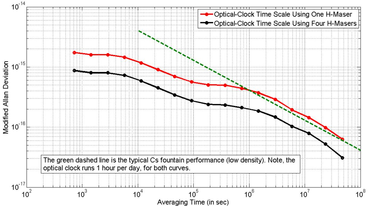
Fig. 8. Simulated results of steering an ensemble of masers to an optical frequency reference that runs 1 h per day. An ensemble of four masers steered to an optical clock running 1 h per day is more stable than a cesium fountain for all averaging times.
