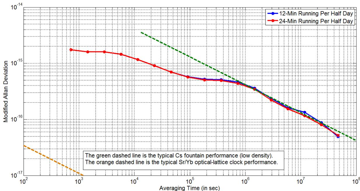
Fig. 4. Running an optical clock every half a day.
