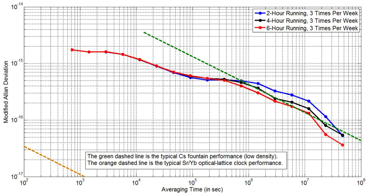
Fig. 6. Running an optical clock 3 times a week.
