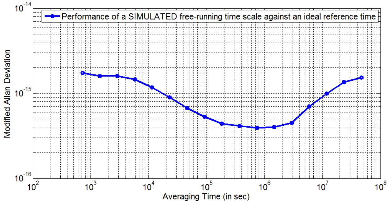
Fig. 2. Frequency stability of a simulated free-running time scale with one maser against an ideal reference time.
