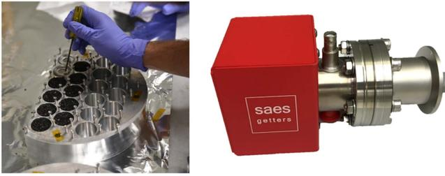
**Figure 5.** Activated getters are used for long-term pressure stability: (a) activated charcoal absorbers being populated in the charcoal getter plate, which is directly mounted to the HPF LN<sub>2</sub> tank; (b) a NexTorr D-100 vacuum pump including an integrated hydrogen getter element and a small ion pump.
