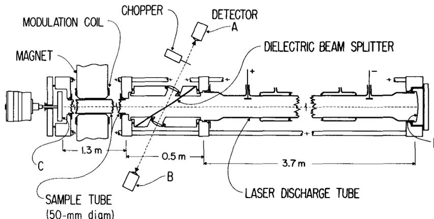
proximately 5 torr. At these pressures the Zeeman components observed were not appreciably power saturated and the linewidths were approximately 1 G. The laser radiation is polarized by the beam splitter and the orientation of the plane of polarization could be made either perpendicular or parallel to the magnetic field  $H_0$  by rotating the entire beam splitter assembly about the laser axis.
