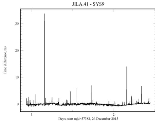
Fig. 4. The time differences, measured every minute, between the free-running clock in system JILA.41 and the remote system SYS9, which was synchronized to UTC. The JILA.41 system had an initial time offset of -270 s and a rate offset of -1.92 s/day, with respect to the remote system, and a straight line with these parameters has been removed from the data in the plot for clarity.
