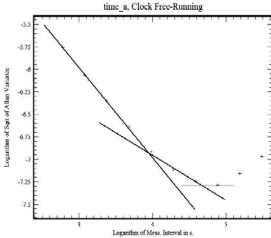
Fig. 1. The two-sample Allan deviation (square root of the Allan Variance) of the free-running stability of the clock in a typical general-purpose computer. The points are the measured time-difference values and the straight lines help to identify the underlying noise types.
