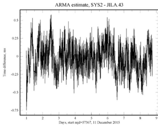
Fig. 3. The time differences between SYS2 and JILA.43 estimated by the auto-regressive process as described in the text. The standard deviation of the data in the figure is 0.22 ms, which is consistent with a mean of zero, confirming the assumption that both systems are independently synchronized to UTC.
