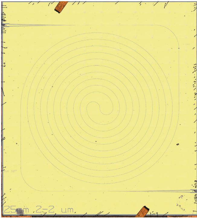
FIG. 1 (color). Photograph of superconducting frequency comb chip. The 25 \mu\text{m} long, \lambda/2 resonator is made in a coplanar waveguide (CPW) geometry with input (output) port at top left (bottom right). The CPW has a 2 \mu\text{m} wide center strip and 2 \mu\text{m} wide gap and is coupled to ports by interdigitated capacitors. The device is made from NbTiN (Au color) on a 2 cm \times 2 cm intrinsic Si ( > 20 k \Omega ) substrate.
