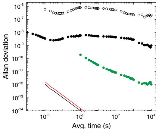
**Fig. 4.** Microcomb optical clock stability. Allan deviation of the DFB lasers (open points) and the microcomb clock (closed black points) normalized to a 33 GHz carrier. The green points are the clock stability after correcting the Rb reference noise via measurements against an auxiliary comb. The red and black traces represent the in-loop residual noise for stabilization of the microcomb pump laser and mode 108, respectively.
