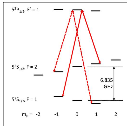
Figure 1. The energy-levels of  $^{87}\text{Rb}$  probed with the double-Lambda lin || lin technique. The two Lambda systems are shown. We use light resonant with the D1 transition at 795 nm.
