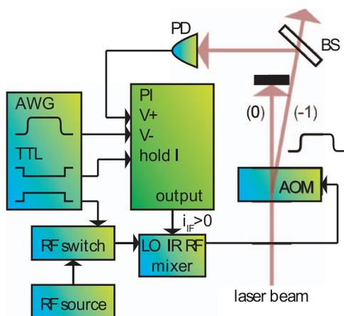
FIG. 7. Laser beam amplitude modulation circuit using a single DAC channel of the AWG, a mixer, and a PI controller in a feedback loop. Feedback is derived from light reflected off of a beam splitter (BS).
