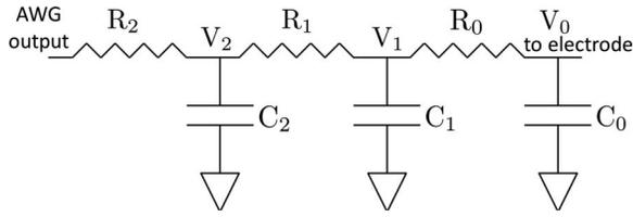
FIG. 5. A diagram of our low-pass RC filter system connected to each electrode. The indices of each passive component correspond to the filter layer, and the voltages correspond to those governed by Eq. (1) with  $V_0$  the final stage applied to the electrode. The values are  $\{R_2, R_1, R_0\} = \{820, 820, 240\} \Omega$  and  $\{C_2, C_1, C_0\} = \{1, 1, 0.82\} \text{ nF}$ .
