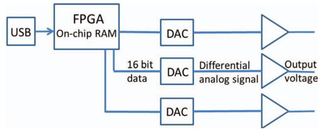
FIG. 2. A flow diagram overview of the AWG. The host computer transmits waveform data via USB to the FPGA, which is stored in on-chip RAM. The FPGA transmits a 16-bit digital signal derived from its RAM to each DAC, whose output is then amplified.
