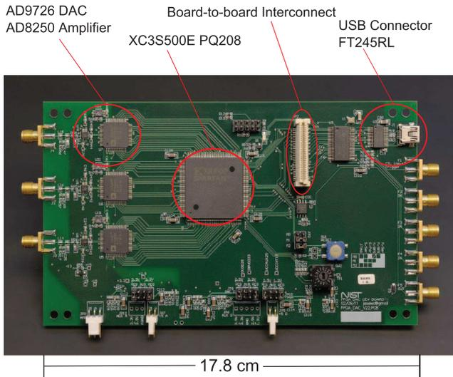
FIG. 3. A master board. The key components described in the text are highlighted. The host computer communicates with the master board via USB. The FT245RL handles the interface with the XC3S500E PQ208 FPGA on up to three boards (a master and two slaves) on a shared communication channel through a board-to-board interconnect. The FPGA drives three AD9726 DACs whose output is fed to AD8250 amplifiers, which creates the final three output potentials.
