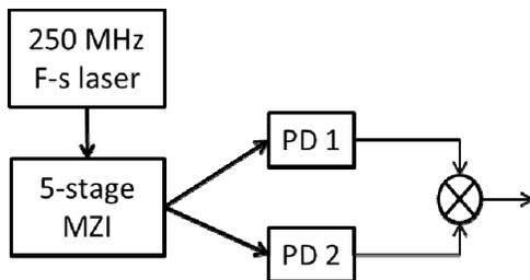
Figure 3. Experimental setup, where MZI is a Mach-Zehnder Interleaver.
