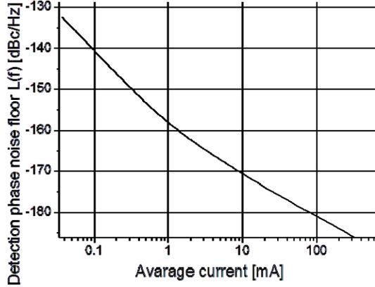
Figure 1. Detection phase noise floor versus average photo-current.
