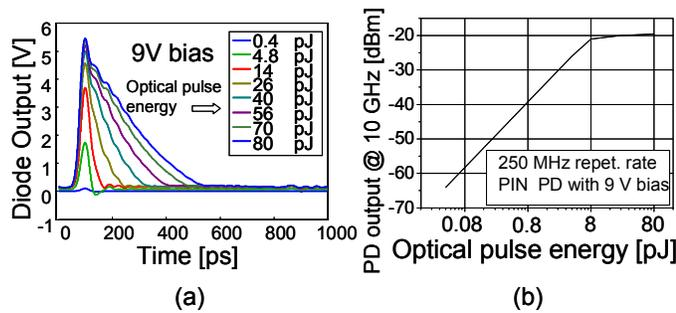
Figure 2. Saturation behavior of a PIN PD, a: time domain PD response and b: frequency domain PD response.
