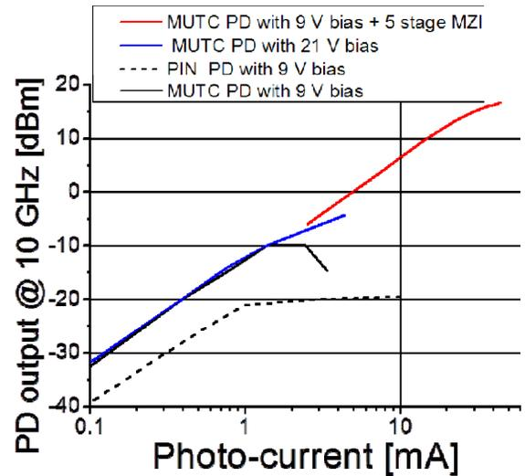
Figure 5. MUTC photodiode output power @ 10 GHz versus photo-current.
