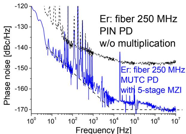
Figure 6. residual photodetection phase noise of a PD with/without multiplier.
