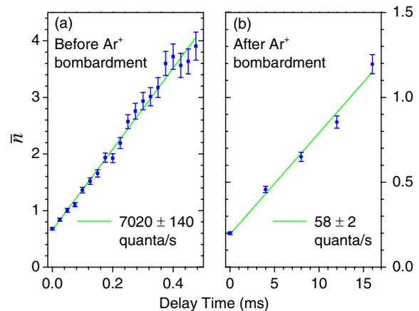
FIG. 3 (color online). Heating rate measurements (a) before and (b) after treatment. Heating rates are obtained by measuring the average number of motional quanta,  $\bar{n}$ , with a variable delay time after initial laser cooling [5].
