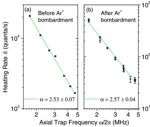
FIG. 4 (color online). Heating rate vs trap frequency, fitted with  $\dot{n} \sim 1/\omega^\alpha$ . The power-law exponents  $\alpha = 2.53 \pm 0.07$  and  $\alpha = 2.57 \pm 0.04$ , (a) before and (b) after treatment in the initial experiments, respectively, are consistent with various adsorbate-induced noise models [4,10–12].
