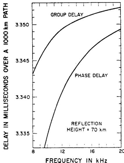
Fig. 1. Phase and group delays of a signal propagated over a 1000-km path as a function of frequency.
