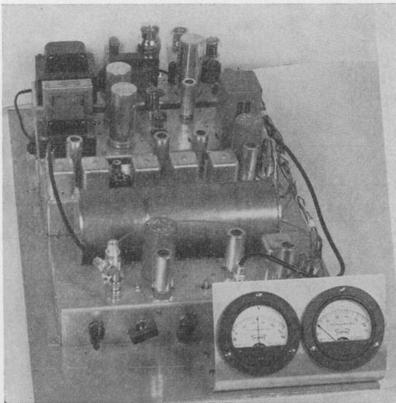
Fig. 7—Photograph of the experimental bridge-balancing oscillator.
