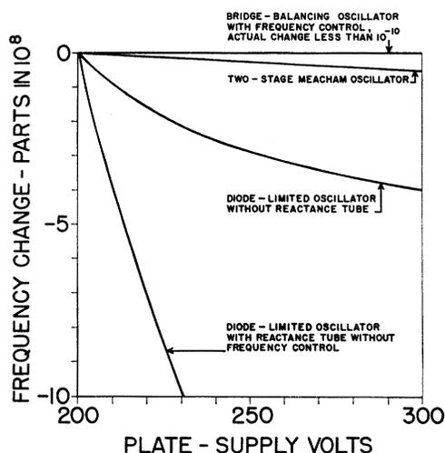
Fig. 2—Frequency change vs plate-supply voltage.
