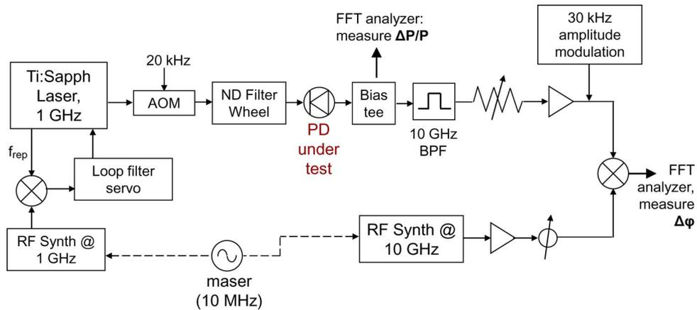
Fig. 3. Block diagram of phase bridge measurement setup.
