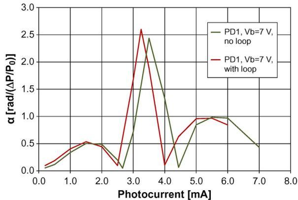
Fig. 8. Phase bridge results for PD1 with changes in shape of the optical mode incident on the detector due to the creation of  $\sim 1$  cm loops in the optical fiber. Note large shifts of nulls and peaks.
