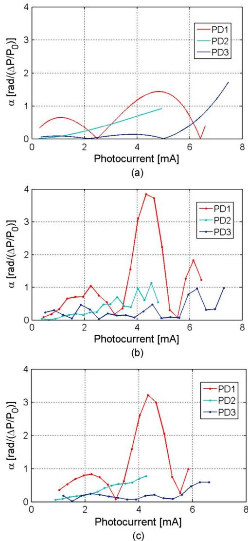
Fig. 7. Compilation of magnitude of  $\alpha$  for the three photodiodes using (a) impulse response with cubic fits, (b) impulse response with point derivatives, and (c) impulse response with triangle filter.
