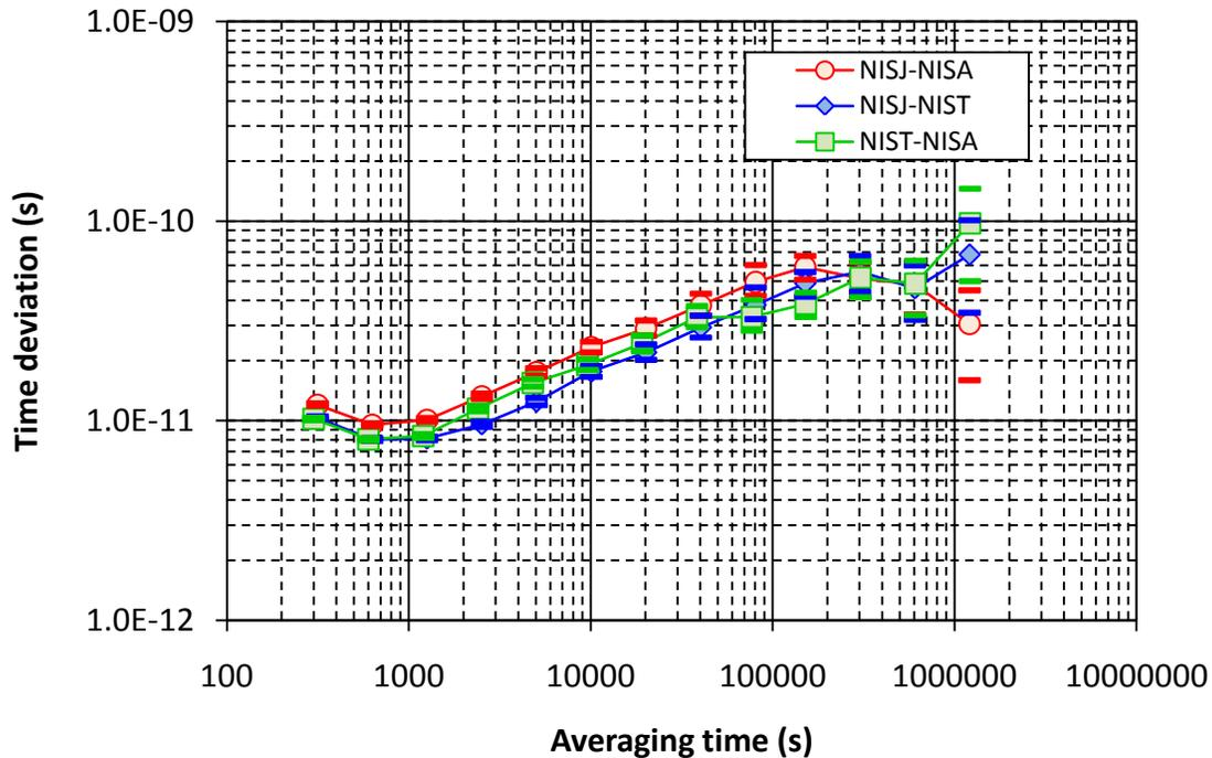
Figure 8. Time deviation of common-clock, TAIPPP differences.
