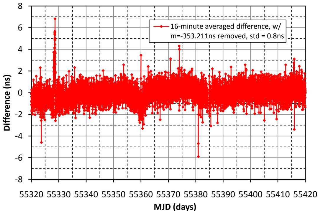
Figure 2. *NISJ - NIST* common-clock, common-view difference.
