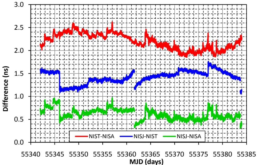
Figure 7. Common-clock, TAIPPP differences (offset for demonstration purposes).
