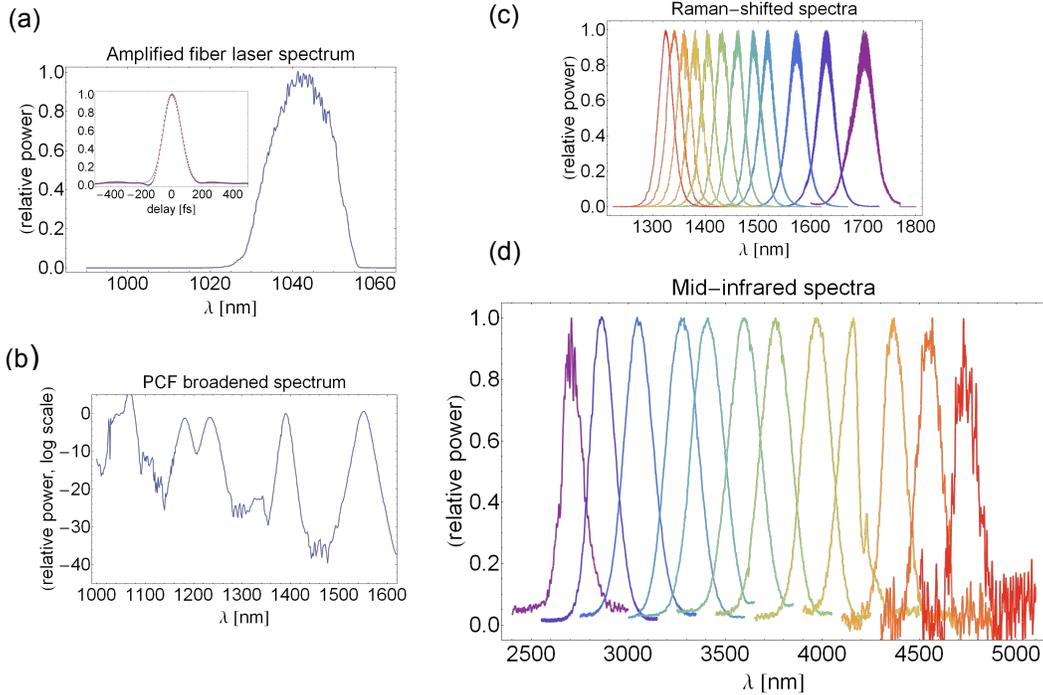
Fig.2. (a) Spectrum from amplified fiber laser, with inset showing ~130fs pulse duration. (b) Broadened spectrum. (c) Raman shifted spectra from PCF. (d) MIR spectra from difference frequency mixing between the amplified laser spectrum and the corresponding Raman peaks from (c).
