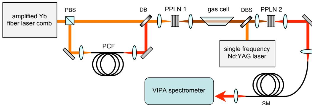
Fig.1. Diagram of the experimental setup. PBS polarizing beam splitter, DBS dichroic beam splitter. PCF photonic crystal fiber, SMF single mode fiber, PPLN periodically poled lithium niobate.
