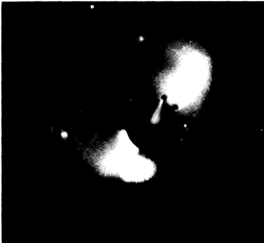
**Stopping sodium atoms** with light. A beam of sodium atoms approaching the camera from the upper right at speeds exceeding 1000 m/sec is brought to a virtual standstill by a laser beam aimed in the opposite direction. In this experiment at NBS, Gaithersburg, the atoms travel down the axis of a solenoid (whose opening appears as the dark circle at the center of the photograph) and spread out as they come to a virtual halt near the opening.<sup>18</sup>
