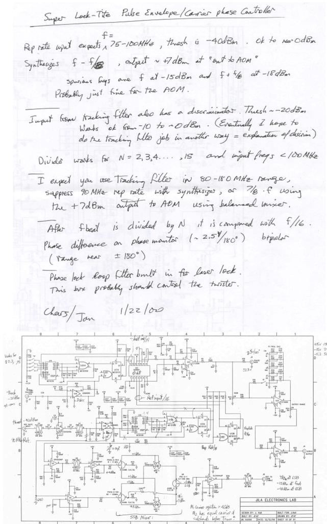
**Figure 4:** The design of the first femtosecond synchronizer stabilizer for the fs comb's offset frequency ( $f_0$ )—the single-wide NIM module that ultimately was called the “femtosecond synchronizer”. His initial thoughts and the resulting design reproduced from our lab books are shown in Fig. 4. True to its name, the femtosecond synchronizer had
