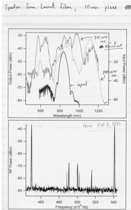
**Figure 1:** Page from lab book on Oct. 6, 1999 showing (top) octave spanning spectrum obtained with Lucent microstructure fiber, and (bottom) the first record of the carrier-envelope offset frequency ( $f_0$ ). Harmonics of the rep rate are at 450 and 540 MHz. Two sweeps of the spectrum analyzer are shown, verifying that  $f_0$  indeed moved with cavity fluctuations (and did it ever move in the open air cavity!) The peak near 515 MHz is spurious.
