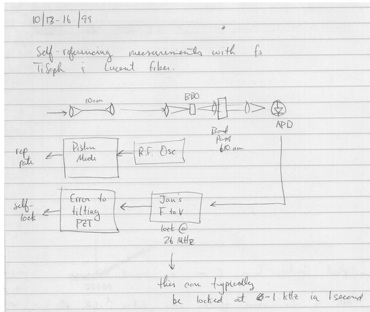
**Figure 2:** (a) Lab book diagram of the initial scheme for measuring and stabilizing  $f_0$ . A split tube piezo transducer in the linear cavity of the femtosecond laser could be driven in two different modes. The piston mode was used to lock the laser repetition rate, while the tilting mode was used to stabilize  $f_0$ . The ideas and hardware for the split piezo and its high voltage driver, the avalanche photodiode (APD), and frequency to voltage converter (F to V) all came from Jan
