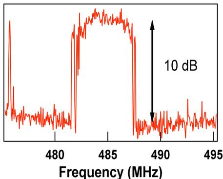
**Figure 3:** On Oct. 16, 1999 we recorded this beat between a tooth of the self-referenced femtocomb (see Fig. 2) and the 2-photon Rb standard at 778 nm.
